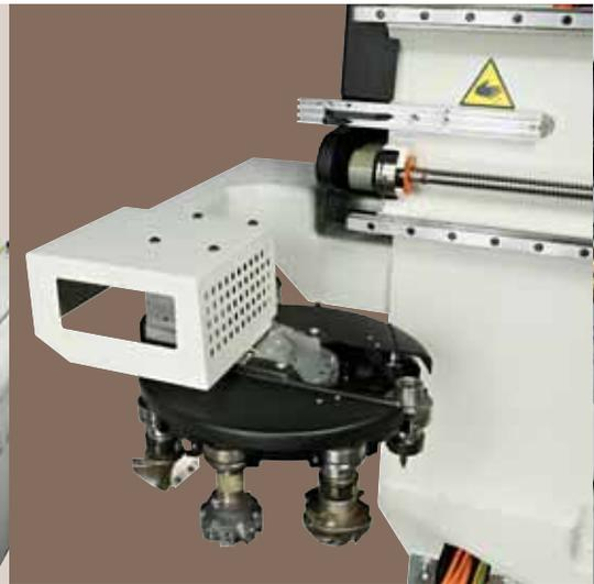
Faster machine tool changeover with the **R8 automatic tool changer mounted** on the Machining Head support beam.
