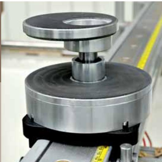
**Mechanical clamps** for securing straight elements for profiling or end trimming.
