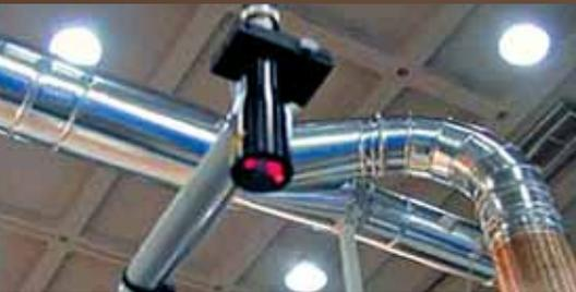
Laser managed by optimisation software for correct positioning of each bar and suction cup.
