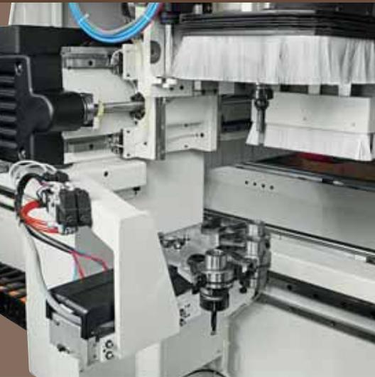
**R4 automatic tool changer** pneumatic with 4 locations mounted on the beam.
