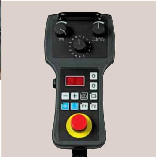
Remote control using **mobile control panel**.
