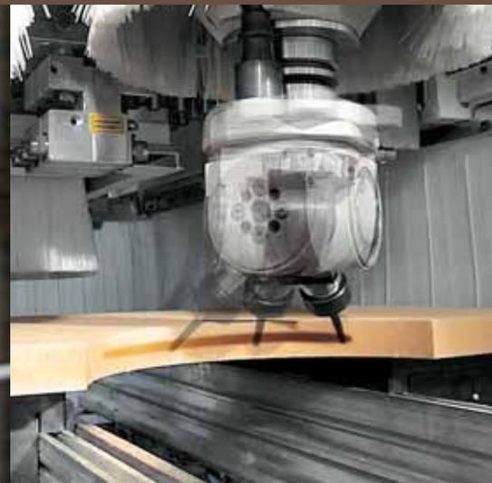
For cutting lock recesses on the rear and routing for hinges on the front using the two-outlet horizontal electro-spindle.
