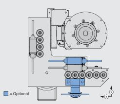
The dimensions of the Y-axis in combination with the compact machining head allow large displacement travels. Large workpieces can be placed very easily.
