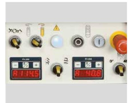
On request, the F 205 can be equipped with powered lifting and tilting of the spindle moulder shaft with digital electronic display of the quotas.
