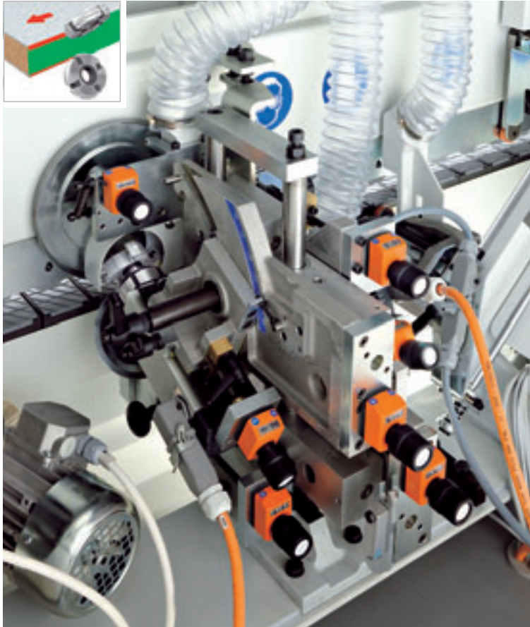
Tilting top and bottom trimming unit RI-501. Two independent high frequency motors (0.65 kW each) which can be tilted from 0 to 25 degrees.
