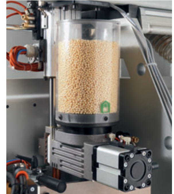
Pre-melting system QM-703 for EVA glue (Optional, not available on Akron 420-425).
