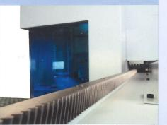
Ensures highest quality and high driving speed up to \*100 m/min in X- and Y-direction
