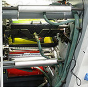
Doctor blade chamber print unit Doctor blade chamber print unit with integrated ink return and drip tray
