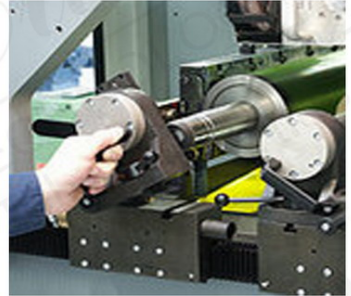
Cantilever bearing Manual hinged bearing
