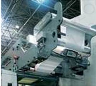
Web aligner and pull roller Web aligner and pull roller at web in-feed
