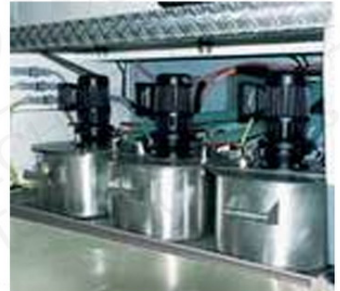
Ink pumps Electrically operated ink pumps
