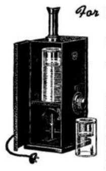
FOR MEASUREMENT OF TURBIDITY (SIO2)
