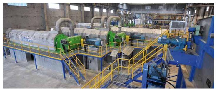
▲ ANDRITZ Screw Presses (SCP1410) as part of a typical four-stage washing system for P-RC APMP.
