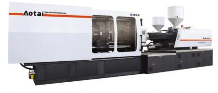
For some special products production, such machine add one set of compound nozzle and feeding barrel assembly on the traditional machine so as to achieve independent double barrels. During injection period, they can achieve double injection by charging with two materials and inject to mold cavity through the conjunct nozzle simultaneous or intervalic, in which the outer charge material is called external material while the inner one is called core material.
