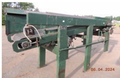
9191 $9,500.00 PENDU SLAB DROP BELT 24" wide x 10' 6" long, hyd drive, twin air cylinders for up-down on belt, heavy duty and in excellent condition 260-633-4047 Wolcottville, IN
