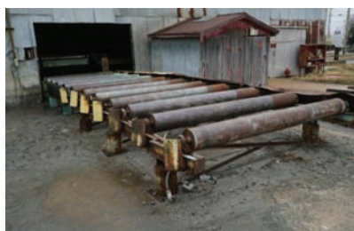
9229 $15,000.00 ROLL CASE 90" wide x 28' long, electric drive, heavy duty and in good condition 260-633-4047 Wolcottville, IN
