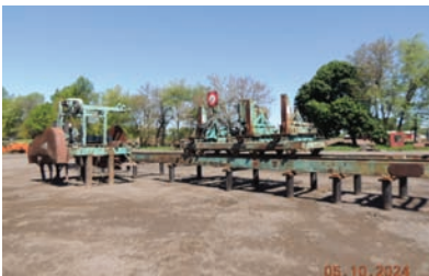
2091 $25,000.00 CIRCLE MILL Helle 3 head block, 36" carriage with 124" knees, husk with top saw, 60' long track, frame, 60 hp carriage drive, cab and all accessories, complete mill ready to work 260-633-4047 Wolcottville, IN
