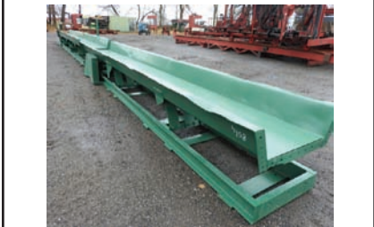
9347 $15,500.00 VIBRATING CONVEYOR 24" wide pan x 46' long, approx 9" tall sides, hyd drive, good working condition 260-633-4047
