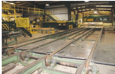
9336 $8,500.00 TRANSFER DECK 5 strand transfer deck, 12' wide x 53' long, H-78 rooftop chain, 15hp electric drive, working condition 260-633-4047
