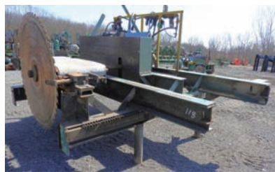
2100 $8,500.00 CLEERMAN CIRCLE SAW HUSK for left hand carriage, includes 56" dia blade in good condition, off-bearer belt is 24" wide x 60" long, includes 200 hp electric motor, unit is in very good condition and ready to work 260-633-4047 Wolcottville, IN
