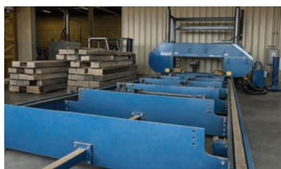
1654 $55,000.00 LQ72 BAKER BAND MILL Industrial slab mill with a 72" wide-cut capacity, ideal for large logs and live-edge slabs. Powered by a 50 HP electric motor with a 5 HP hydraulic system. 3-phase power required. Features include hydraulic variable-speed feed, dual-chain forward/reverse drive, and a heavy twin I-beam frame. Bed 20' long. Capable of cutting logs up to 20' long. This is a stationary mill (not trailer portable). Loading is available. Call for details. Or best offer! 831-768-3880
