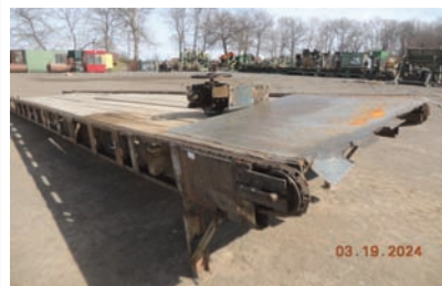
9169 $5,250.00 GREEN CHAIN 2 strand green chain, 5' 6" wide x 32' long, gearbox drive, C-55 rooftop chain, good working condition 260-633-4047 Wolcottville, IN
