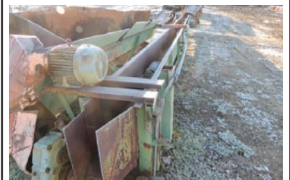
9142 WASTE CONVEYOR $8,500.00 10"x60' waste conveyor H78 chain with paddles, electric drive .includes new chain 260-633-4047
