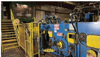
5136 $45,000.00 EDGER Timber Machine Technologies heavy duty edger, 8" thick x 38" wide capacity, 400 hp electric drive motor, bottom splined arbor, includes operating cab and all controls, ready for production 260-633-4047
