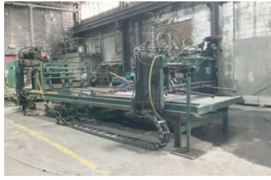
14092 PALLET NAILER $32,500.00 Viking Champion 304, 4 stringer capacity, 60" x 78" pallet capacity, includes auto pallet stacker, good working condition and recently in production 260-633-4047
