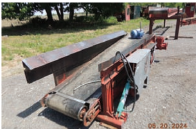
9180 DROP BELT $6,500.00 Slab drop belt, 24" wide x 12' long, electric drive, hyd cylinder for drop belt, includes hyd unit for cylinder, very good condition 260-633-4047
