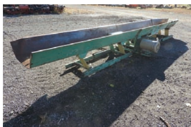
9240 WEBSTER VIBRATING CONVEYOR $7,500.00 18" wide pan x 20' long, electric drive, good working condition 260-633-4047
