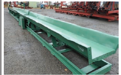
9347 VIBRATING CONVEYOR $15,500.00 24" wide pan x 46' long, approx 9" tall sides, hyd drive, good working condition 260-633-4047
