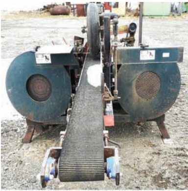
6045 RING DEBARKER $57,500.00 30" dia Cambio ring debarker, 6 arms, steel infeed press wheels, all electric, all electrical and controls included, recently in production and in good working condition, infeed/ outfeed also available, call for price 260-633-4047
