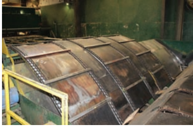
9337 UNSCRAMBLER $8,500.00 6 strand unscrambler, approx 60" tall, electric drive, good working condition 260-633-4047
