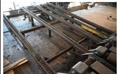
9018 TRANSFER DECK $4,600.00 5 strand, 13' wide x 18' 6" long, H78 chain, electric drive, air cylinders on pop up board stop, good condition 260-633-4047
