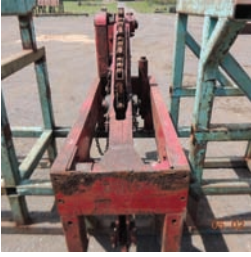
8057 LOG TURNER $3,500.00 36" chain type log turner, hyd drive, good working condition 260-633-4047
