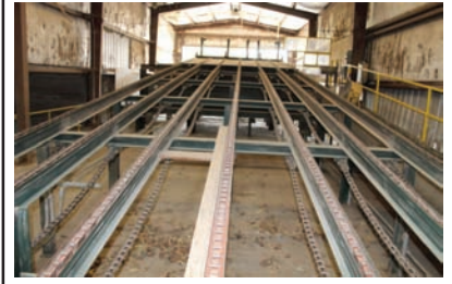
9344 TRANSFER DECK $7,500.00 7 strand transfer deck, 12' wide x 45' long, 81X chain, electric drive, good working condition 260-633-4047
