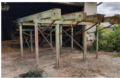
9357 TRANSFER DECK $3,750.00 4 strand transfer deck, 10' wide x 15' long, electric gearbox drive, H-78 chain, good condition 260-633-4047
