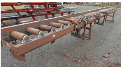
9348 ROLL CASE $2,500.00 14" wide x 25' long, 4" dia rollers, rolls spaced every 8", hyd drive, good working condition 260-633-4047
