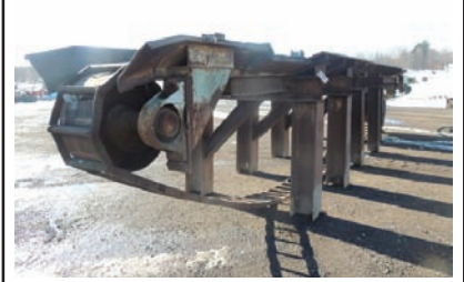
9090 LOG TROUGH $14,300.00 40' long, 110 ladder-back chain, 14" wide, s- style drive, no power, good working condition 260-633-4047
