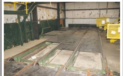
9335 TRANSFER DECK $7,500.00 10' wide x 40' long, H-78 chain, electric gear-box drive, includes panning in between strands, very good condition 260-633-4047
