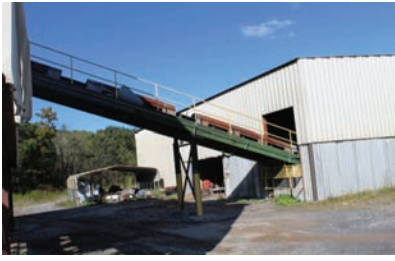
9342 WASTE BELT CONVEYOR $11,500.00 concave style belt conveyor, 24" wide x 65' long, electric drive, includes cat-walk on side, excellent condition 260-633-4047
