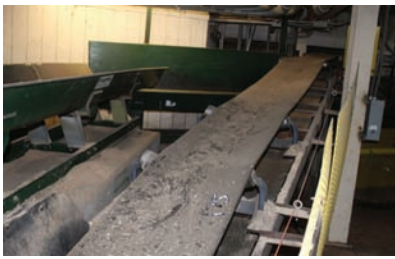
9339 WASTE BELT CONVEYOR $4,500.00 concave style belt conveyor, 20" wide x 22' long, electric drive, very good condition 260-633-4047
