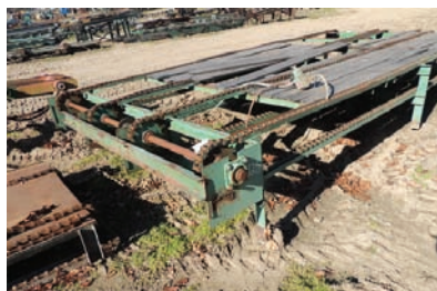
9249 TRANSFER DECK $5,000.00 4 strand, 10' wide x 22' long, H-78 chain, good condition 260-633-4047
