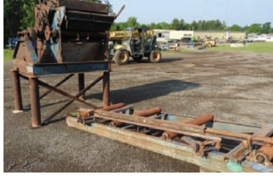
5134 $10,500.00 EDGER Cornell edger 6" thick x 36' wide capacity, 1 stationary-2 movable blades, air-powered hold-downs, includes 8' long infeed rollers, movable fence, working condition 260-633-4047
