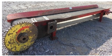
9309 BELT CONVEYOR $1,250.00 16" wide x 7' long, 4" tall sides, no power, good condition 260-633-4047
