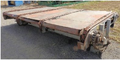
9316 TRANSFER DECK $3,750.00 4 strand transfer deck, approx 9' wide x 8' long, H-78 rooftop chain, electric drive, good condition 260-633-4047
