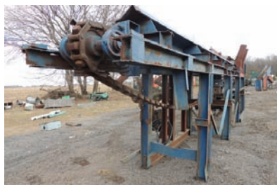
9232 LOG TROUGH $17,250.00 chain is 11" wide, trough is 38' long, electric gear box drive, 1 set of kickers, heavy duty and in good condition 260-633-4047
