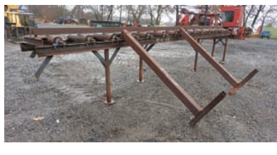
9349 ROLL CASE $2,500.00 16" wide x 19' long, 4 1/2" dia rollers, dead rolls, roll spacing 11", good working condition 260-633-4047
