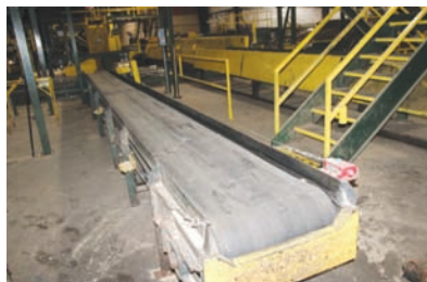
9334 BELT CONVEYOR $4,500.00 24" wide x 30' long, electric drive, 4" tall sides, excellent condition 260-633-4047
