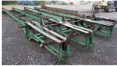
9321 LOG DECK $10,500.00 Edmiston log deck, 4 strands 12' wide x 34' long H-78 chain, stop-load, good working condition 260-633-4047
