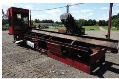
6046 DEBARKER $42,500.00 Mellott rosser-head debarker, your choice of power (electric or hyd), new babbit in bearings, new cleats on bull wheels, good condition and ready for production 260-633-4047
