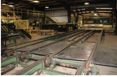
9336 TRANSFER DECK $8,500.00 5 strand transfer deck, 10' wide x 55' long, H-78 chain, electric drive, good working condition 260-633-4047
