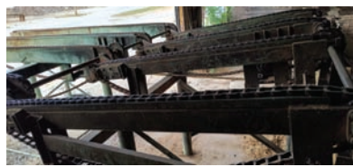
9358 TRANSFER DECK $3,250.00 4 strand transfer deck, 10' wide x 10' long, H-78 chain, electric gearbox drive, good condition 260-633-4047
