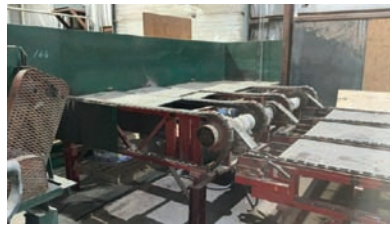
9355 TRANSFER DECK $4,500.00 4 strand transfer deck, 8' wide x 12'-6" long, H-78 rooftop chain, electric drive, good condition 260-633-4047
