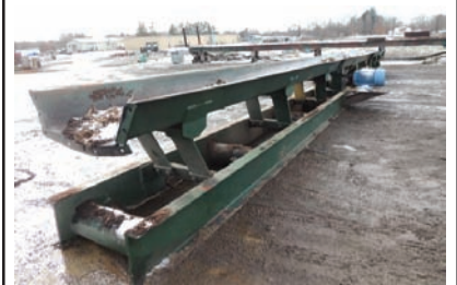
9119 VIBRATING CONVEYOR $13,750.00 Jeffrey vibrating conveyor, 18" wide pan x 36' long, 6" tall sides, electric drive, good working condition 260-633-4047
