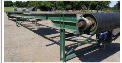
9305 BELT CONVEYOR $9,500.00 60" wide x 50' long ,electric drive, no sides, good working condition 260-633-4047
