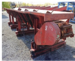
9327 MELLOTT LOG TROUGH $14,500.00 ladder-back chain, includes air-powered kickers, hyd drive, very good condition 260-633-4047
