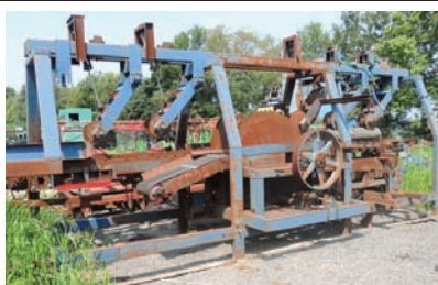
19008 $86,250.00 SCRAGG MILL Fast Line scragg mill, similar to "Big Jake", twin blades 56" dia, electric drive, includes off-bearer belts, price includes controls and machine gone through shop, ready for production 260-633-4047 Wolcottville, IN
