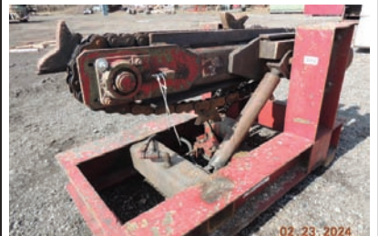
8054 MELLOTT 6 LOG TURNER Mellott #6 chain type 48" Log Turner (Sawmill), all hyd, working condition 260-633-4047
