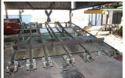
9383 $5,500.00 TRANSFER DECK 6 strand transfer deck, 10' 6" wide x 16' long, C-55 rooftop chain, electric drive, good working condition 260-633-4047
