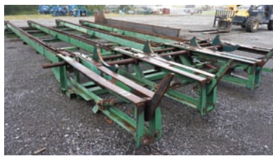
9321 $10,500.00 EDMISTON LOG DECK 4 strands 12' wide x 34' long H-78 chain, stop-load, good working condition 260-633-4047
