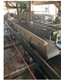
9243 DROP BELT CONVEYOR $7,200.00 Reckart drop belt, 24" wide x 13' long, air cylinder for up-down, hyd drive, good working condition 260-633-4047
