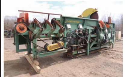
17099 $27,500.00 MERCHANDISING SAW Compact Maxi-Tour merchandising saw system, 72" dia blade, 75 hp electric drive, includes infeed/outfeed conveyors 260-633-4047 Wolcottville, IN
