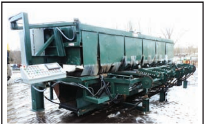
17128 $75,000.00 DROP SAW TRIMMER Sanborn drop saw trimmer, 9 saws, 4'-16' capacity, odd-length blade, computerized controls, automatic length function, hyd drive on heads, excellent condition and ready for production 260-633-4047
