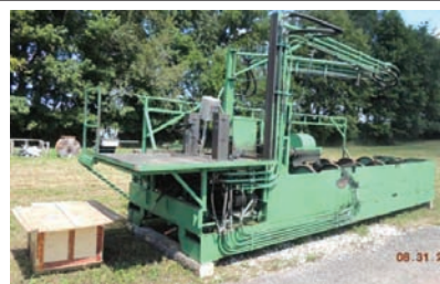
6031 $34,500.00 HMC DEBARKER rosser head style, all hyd. drive, 36" dia. log capacity x 12' long, very good condition 260-633-4047
