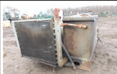
18184 $2,300.00 HYD UNIT pressure comp pump, has reservoir and cooling radiator 260-633-4047
