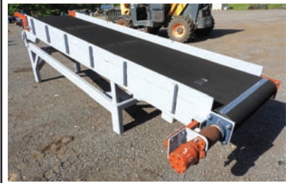
9298 $12,500.00 SLAB DROP BELT 34" wide x 12' long, hyd drive, hyd cylinder for up-down movement, brand new and ready for production 260-633-4047
