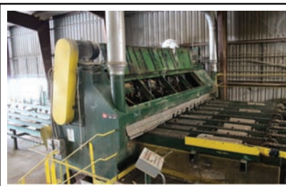
17127 $45,000.00 DROP SAW TRIMMER Newnes drop saw trimmer, 16' long capacity, 9 saws, 7 5 hp electric motor single drive unit for all saws, easy to set up for line-shaft, air power for heads up/down movement, includes infed deck/ even-end rollers, includes control station, good working condition 260-633-4047
