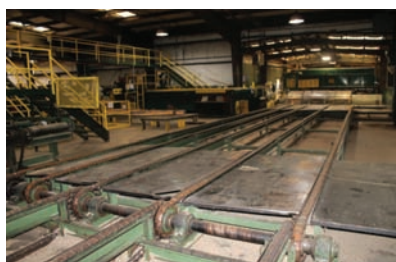
9336 $8,500.00 TRANSFER DECK 5 strand transfer deck, 12' wide x 53' long, H-78 rooftop chain, 15hp electric drive, working condition 260-633-4047
