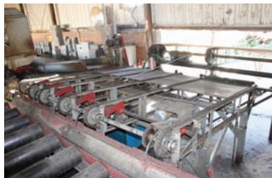
9382 $3,750.00 TRANSFER DECK 6 strand transfer deck, 10' 6" wide x 11' long, C-55 rooftop chain, electric drive, air stops on one end, good working condition 260-633-4047
