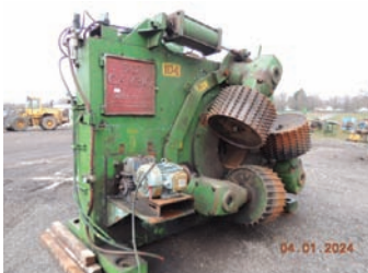
6045 $57,500.00 RING DEBARKER 30" dia Cambio ring debarker, 6 arms, steel infeed press wheels, all electric, all electrical and controls included, recently in production and in good working condition, infeed/ outfeed also available, call for price 260-633-4047
