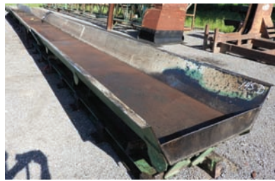
9296 $22,500.00 PRECISION VIBRATING CONVEYOR 30" wide pan x 58' long, 12" tall sides, hyd drive, excellent condition 260-633-4047
