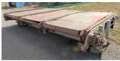
9316 $3,750.00 TRANSFER DECK 4 strand transfer deck, approx 9' wide x 8' long, H-78 rooftop chain, electric drive, good condition 260-633-4047
