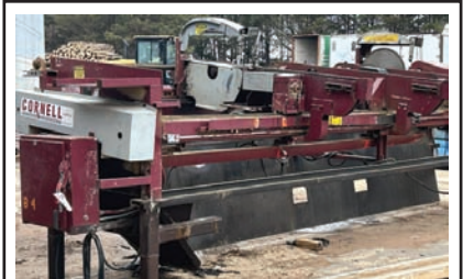
17613 $11,500.00 CORNELL 2 BLADE TRIM SAW 1993 model, equipped with 10 HP motors on each movable blade. Includes 3 HP hydraulic power pack, machine control center, operator controls, and 4 blades. Ready to run. Call for details. Make your offer today! 906-295-0545
