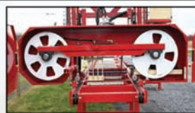
ROCK SOLID FRAMEWORK • 30" BAND WHEELS • 2" BAND • 120 HP DIESEL OR • 60HP ELECTRIC
