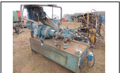
18186 $5,000.00 HYDRAULIC PACK 30 HP electric motor w/double pump direct mounter, approx. 100 gal tank, lots of electric control valves, oil cooler, electric control box 260-633-4047
