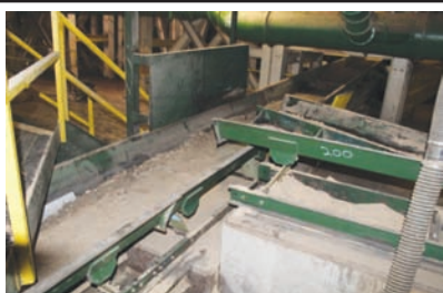
9340 $19,500.00 PROGRESS VIBRATING CONVEYOR 24" wide pan x 55' long, 9" tall sides, 15 hp electric power unit, working condition 260-633-4047
