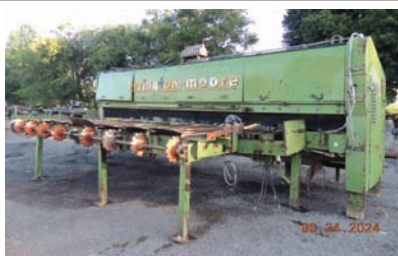
17112 $17,500.00 DROP TRIMMER 9 blades, up to 18' long capacity, air cylinders on heads, electric powered, price does not include going through shop 260-633-4047 Wolcottville, IN
