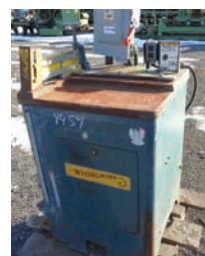
17118 $2,750.00 CHOP SAW Whirlwind up-cut chop saw, 2-3/16" x 8-1/4" cutting capacity, electric drive, air power for blade movement, good working condition 260-633-4047 Wolcottville, IN
