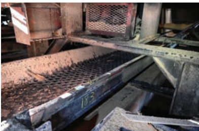
9381 $10,500.00 WEBSTER VIBRATING CONVEYOR 18" wide pan x 30' long, 6" tall sides, electric drive, sawdust/ fines section, good working condition 260-633-4047
