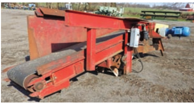
9291 $6,500.00 DROP BELT CONVEYOR 24" wide x 11' long, electric drive, air cylinder for up-down movement, good working condition 260-633-4047
