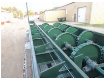
6048 $87,500.00 DEBARKER Precision rosser head debarker, Model P636, Serial # D563, 36" capacity, electric drive on head, self-contained hyd unit for carriage etc., upgraded to chain drive for carriage, price is Showase Rebuilt and comes with warranty. CURRENTLY IN THE SHOP SO CALL WITH YOUR SPECS TO HAVE IT CUSTOMIZED! pics similar to actual machine 260-633-4047
