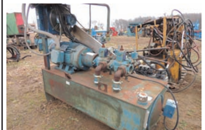
18186 $5,000.00 HYDRAULIC PACK 30 HP electric motor w/double pump direct mounter, approx. 100 gal tank, lots of electric control valves, oil cooler, electric control box 260-633-4047 Wolcottville, IN
