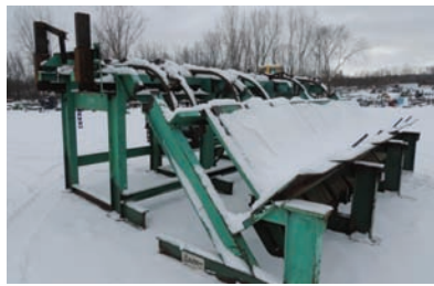
9121 $9,750.00 UNSCRAMBLER Irvington-Moore 7 strand unscrambler, 75" tall, includes even-end rollers, electric drive, good working condition 260-633-4047
