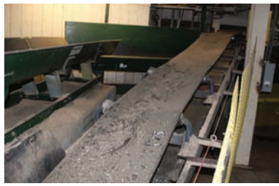
9339 $4,500.00 WASTE BELT CONVEYOR concave style belt conveyor, 20" wide x 24' long, electric drive, good condition 260-633-4047
