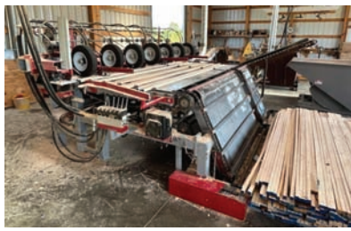
17618 $30,000.00 CUSTOM BUILT 8 BLADE CHOPSAW 8-blade system designed to self-feed lumber through the saw blades, then drop the cut pieces onto a transfer belt. Also equipped with an unscrambler for efficient material handling. A complete setup built for production. Call for details and make your offer today! 270-465-0505 Campbellsville, KY
