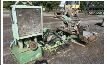
18239 CARRIAGE DRIVE $3,500.00 Tyrone-Berry carriage drive, includes valve for sawyer, good working condition 260-633-4047
