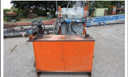
18254 HYD UNIT $5,000.00 30hp. pressure comp hyd pack, approx. 95 gal. capacity, includes heat exchanger, electrical box, and various valves, excellent condition 260-633-4047
