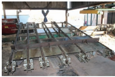
9383 $5,500.00 TRANSFER DECK 6 strand transfer deck, 11' wide x 16' long, C-55 rooftop chain, bottom height 2', top height 4'6", electric drive, good working condition 260-633-4047
