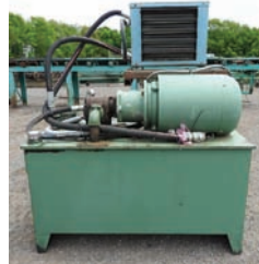
18246 HYD POWER UNIT $3,500.00 40 hp electric, vane type pump, includes cooling radiator, approx. 120 gallon capacity, good working condition 260-633-4047
