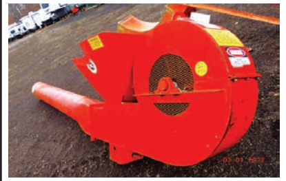
10211 $3,450.00 MORBARK CHIP BLOWER 30 in. dia. 15 HP. electric motor, includes mounting plate and pipe, VERY GOOD CONDITION 260-633-4047 Wolcottville, IN
