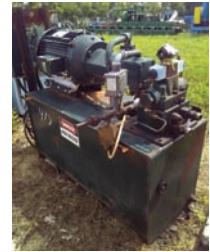
18247 HYD POWER UNIT $2,500.00 20 hp electric drive hyd power unit, gear style pump, approx 40 gal reservoir, includes control panel, good working condition 260-633-4047
