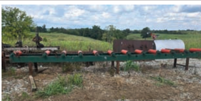
9633 $3,000.00 HEAVY DUTY ROLLCASE 24" wide x 25' long, equipped with 6" rollers. No power unit included. Heavy-built rollcase ready to be powered to fit your operation. Call for details and make your offer today! 502-905-1940
