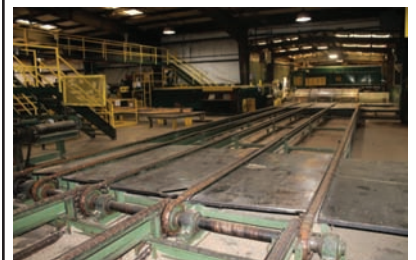
9336 $ 8,500.00 TRANSFER DECK 5 strand transfer deck, 10' wide x 55' long, H-78 chain, electric drive, good working condition 260-633-4047
