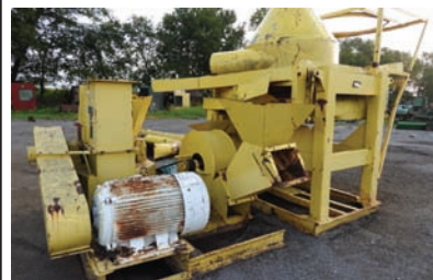
7154 CHIP-PAC $ 22,500.00 Fulghum 48" dia chipper, 3 knives, 150 hp electric drive, 5' x5' shaker screen-electric drive, chip blower-electric drive, complete unit that is in good condition and ready to work 260-633-4047
