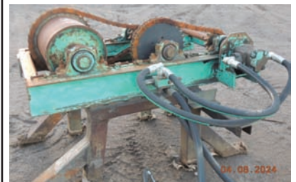
20308 $ 2,800.00 CARRIAGE DRIVE Helle cable drum unit for carriage drive, drum is 13 1/2" dia x 16" wide, hyd drive, good working condition 260-633-4047
