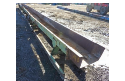
9226 $ 15,000.00 VIBRATING CONVEYOR Precision vibrating conveyor, 18" wide pan x 55' long, 8" sides, electric drive, good working condition 260-633-4047
