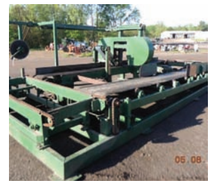
3087 $ 40,000.00 GRADE RESAW "Hochstetler" band resaw, 12" x12" x 12' long capacity, 2" x 30" band wheels, line-shaft ready, foot print 11'6" wide x 28'6" long, complete run-around system ready to work, very good condition 260-633-4047 Wolcottville, IN
