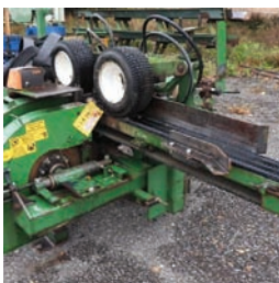
3103 $ 21,500.00 RESAW Morgan double head resaw with return, lineshaft ready, upgraded to guide rollers, recently in production, good condition 260-633-4047 Wolcottville, IN
