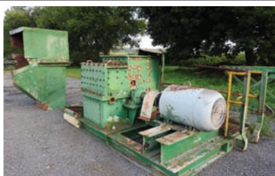
7155 WASTE GRINDER $ 8,500.00 Progress waste grinder, swinging hammer style, 125 hp electric drive, 1185 rpm's, unit needs to have hammers installed, good overall condition 260-633-4047
