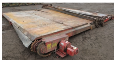
9220 $ 8,500.00 SLAB DRAG DECK slab drag, 15' x 15', electric gearbox drive, 81X chain with steel cleats bolted on, good working condition 260-633-4047
