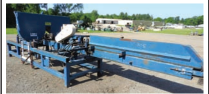
3093 $ 15,000.00 RESAW Brewer Golden Eagle single head resaw, electric drive, 36" dia wheels, return belt, includes numerous extra blades, this machine is in excellent condition and ready for production 260-633-4047 Wolcottville, IN
