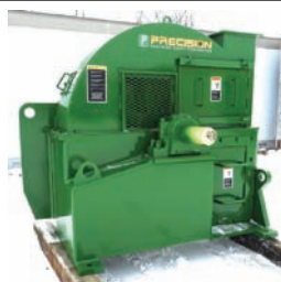
7159 CHIPPER $ 81,247.00 Precision 58" dia, 6 knife, hard surfaced anvils, Kwik-Change knife system, THIS UNIT IS BRAND NEW!! in-stock and ready to ship 260-633-4047
