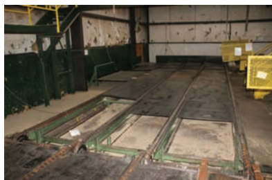
9335 $ 7,500.00 TRANSFER DECK 10' wide x 40' long, H-78 chain, electric gear-box drive, includes panning in between strands, very good condition 260-633-4047
