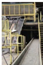
9338 $ 6,500.00 BELT CONVEYOR 24" wide x 77' long, approx 6" tall sides, electric drive, good working condition 260-633-4047
