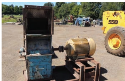
7134 WASTE GRINDER $ 6,300.00 Roberts hammer mill/ waste grinder, 1/4" screen, top feed, 60 hp electric drive, 3600 rpm's, good working condition 260-633-4047
