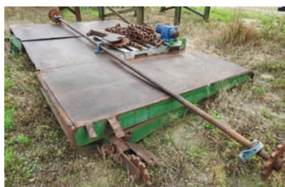
9223 $ 8,500.00 SLAB DRAG DECK slab drag conveyor, 15' x 14', electric gearbox drive, 81X chain with steel cleats bolted on, good condition 260-633-4047
