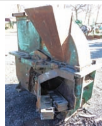
7161 CHIPPER $ 12,500.00 PHL Industries 48" dia chipper, 6 knife wheel with 3 blocked, includes some spare knives, good working condition 260-633-4047
