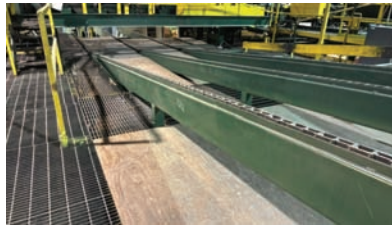
9350 $10,500.00 TRANSFER DECK 3 strand transfer deck, 8' wide x 62' long, 81X chain, electric drive, heavy duty and in good condition 260-633-4047
