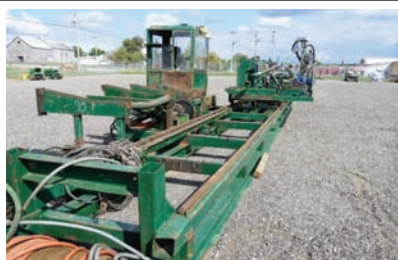
2087 $20,000.00 HMC 4 HEAD BLOCK CARRIAGE HMC HC-40, serial #330-1982, 4 head-block carriage, 110 volt electric over air set-works, 50 hp carriage drive, air powered dogs, 40' long track, was used with band head, includes cab, controls and log turner, complete unit ready to operate and in good condition 260-633-4047
