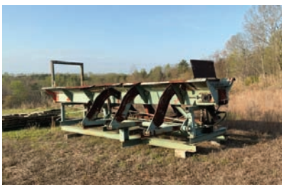
9384 MORBARK LOG TROUGH $22,500.00 110 ladderback chain, 2- way log kickers, 26' long over-all, hyd powered, good working condition 260-633-4047
