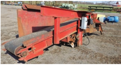
9291 $6,500.00 DROP BELT CONVEYOR 24" wide x 11' long, electric drive, air cylinder for up-down movement, good working condition 260-633-4047
