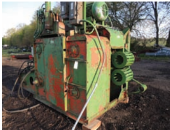
6042 $25,500.00 RING DEBARKER Valone Kone ring debarker, electric drive, includes infeed/outfeed, working condition 260-633-4047
