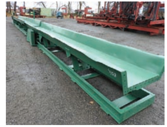
9347 $15,500.00 VIBRATING CONVEYOR 24" wide pan x 46' long, approx 9" tall sides, hyd drive, good working condition 260-633-4047
