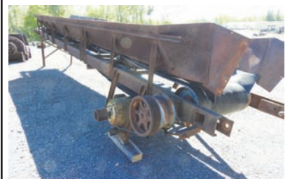
9325 $4,500.00 BELT CONVEYOR concave style belt conveyor, 30" wide x 27' long, electric drive, working condition 260-633-4047
