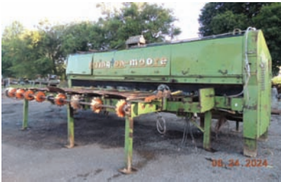
17112 $17,500.00 DROP TRIMMER 9 blades, up to 18' long capacity, air cylinders on heads, electric powered, price does not include going through shop 260-633-4047
