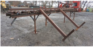
9349 $2,500.00 ROLL CASE 16" wide x 19' long, 4 1/2" dia rollers, dead rolls, roll spacing 11", good working condition 260-633-4047
