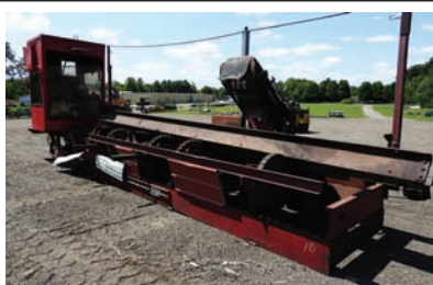
6046 $42,500.00 DEBARKER Mellott rosser-head debarker, your choice of power (electric or hyd), new babbit in bearings, new cleats on bull wheels, good condition and ready for production 260-633-4047
