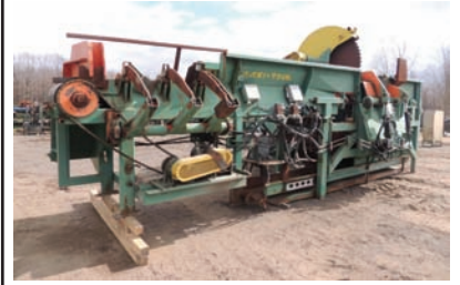
17099 $27,500.00 MERCHANDISING SAW Comact Maxi-Tour merchandising saw system, 72" dia blade, 75 hp electric drive, includes infeed/outfeed conveyors, 260-633-4047
