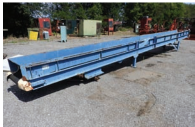
9389 BELT CONVEYOR $4,000.00 24" wide X 30' long belt conveyor, approx. 10" sides, electric gear box drive, good condition 260-633-4047
