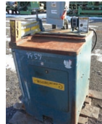
17118 $2,750.00 CHOP SAW Whirlwind up-cut chop saw, 2-3/16" x 8-1/4" cutting capacity, electric drive, air power for blade movement, good working condition 260-633-4047
