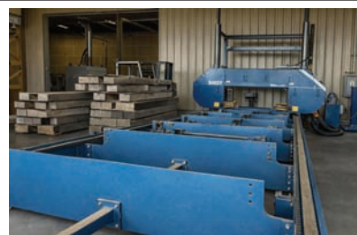
1654 $55,000.00 LQ72 BAKER BAND MILL Industrial slab mill with a 72" wide-cut capacity, ideal for large logs and live-edge slabs. Powered by a 50 HP electric motor with a 5 HP hydraulic system. 3-phase power required. Features include hydraulic variable-speed feed, dual-chain forward/reverse drive, and a heavy twin I-beam frame. Bed 20' long. Capable of cutting logs up to 20' long. This is a stationary mill (not trailer portable). Loading is available. Call for details. Or best offer!
