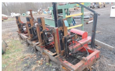
2072 $11,500.00 MEADOWS MILL Meadows 4 headblock carriage, Model; #3 DELUXE, 40" long track, was used with band head, good working condition 260-633-4047
