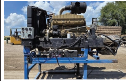
12661 $8,000.00 CUMMINS DIESEL POWER UNIT 350 HP Cummins diesel power unit with Allison transmission. Hours are unknown. Needs a new battery, and the third gear in the transmission is not working. A good repair project or source for parts. Call for details. Make your offer today! 641-895-2872 Seymour, IA.
