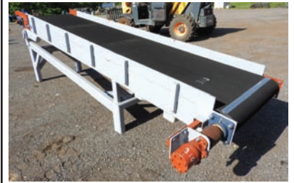
9298 $12,500.00 SLAB DROP BELT 34" wide x 12' long, hyd drive, hyd cylinder for up-down movement, brand new and ready for production 260-633-4047
