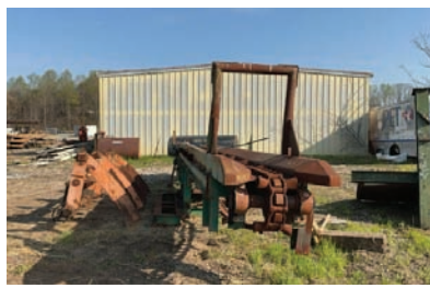
9385 LOG TROUGH $15,500.00 31' long over-all, S-style drive construction, includes log kickers, working condition 260-633-4047
