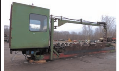
6044 $34,500.00 DEBARKER Mellott rosser-head debarker, electric drive, hyd cylinder for head up-down, recently in production and in good operating condition 260-633-4047
