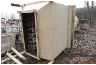
10309 BAG HOUSE SYSTEM $4,000.00 Honeyville Metal baghouse is approx. 8' x 8', 72 - 5" x 60" bags, 11" x 13" inlet, 28" x 63" bottom outlet, includes blower and numerous pipes, good condition 260-633-4047
