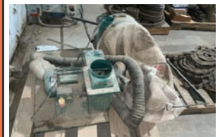
Grizzly Dust Blower and Collection Bag — Specifications & Features — Make: Grizzly. Model: na. Serial #: na. Drive Type: Electric. Inlet Size: 2 way split adapter: 3 1/2". Outlet Size: 4 1/2". Size: 18". — Seller Statement — Includes short flex hose, powered by 1.5 hp electric motor Eligible for free loadout
