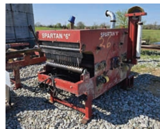
4606 $12,000.00 MEADOWS 6" SPARTAN GANG / EDGER Includes 9' infeed and 9' outfeed, plus 9 replacement blades. Equipped with laser light, 2-blade edger (1 movable blade) on the right side, and gang on the left side. 15" board width capacity on both sides. In good condition. Call for details. Make your offer today! 502-905-1940
