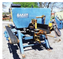
3109 $12,500.00 RESAW Baker single head resaw with turn table return, 670cc Predator gas motor, hyd variable feed drive, block guides, good working condition 260-633-4047 Wolcottville, IN
