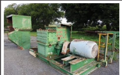
7155 $8,500.00 WASTE GRINDER Progress waste grinder, swinging hammer style, 125 hp electric drive, 1185 rpm's, unit needs to have hammers installed, good overall condition 260-633-4047
