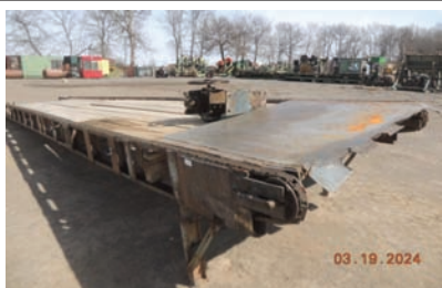
9169 $5,250.00 GREEN CHAIN 2 strand green chain, 5' 6" wide x 32' long, gearbox drive, C-55 rooftop chain, good working condition 260-633-4047
