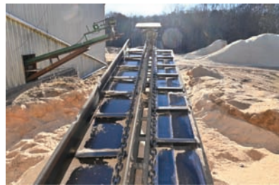
10394 $8,500.00 WASTE CONVEYOR Cornell style chain bran sweep, 14" wide paddles, 27' flat section, 30' long incline section, electric drive, good working condition 260-633-4047 Wolcottville, IN
