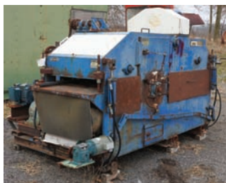
4042 $30,000.00 GANG SAW Quality Machine single arbor gang saw, 6" thick x 24" wide capacity, has indexable sizer head, waste belt, all electric drive, 100hp, 25hp, and 10hp motors, 10 blades and lots of various spacers, has 6' in feed, good working condition 260-633-4047
