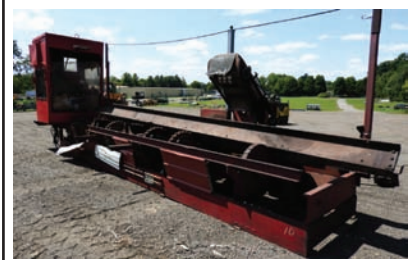
6046 DEBARKER $42,500.00 Mellott rosser-head debarker, your choice of power (electric or hyd), new babbit in bearings, new cleats on bull wheels, good condition and ready for production 260-633-4047
