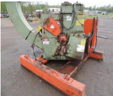
6046 DEBARKER $42,500.00 Mellott rosser-head debarker, your choice of power (electric or hyd), new babbit in bearings, new cleats on bull wheels, good condition and ready for production 260-633-4047
