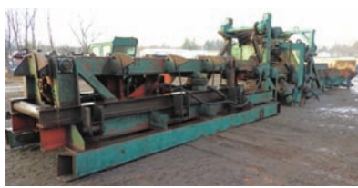
6047 DEBARKER $55,000.00 30" Cambio 5 arm ring debarker, electric drive, includes infeed/ outfeed log troughs and all controls, in good condition and ready for production 260-633-4047
