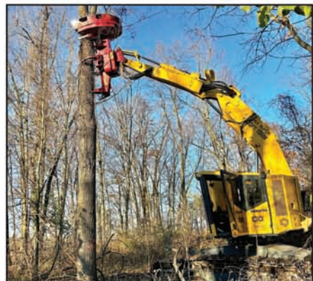
Scoring a Walnut crotch to keep it from splitting the log when it hits the ground.
