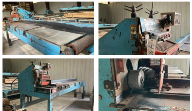
Hasko Power Feeder — Specifications & Features — Make: Hasko. Model: HSFF. Serial #: 0443704. — Seller Statement — Part of entirety Power feeder for side matcher or molder. 20" x 13' , hyd driven, includes hydraulic Pak. Eligible for free loadout
