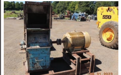
7134 $6,300.00 WASTE GRINDER Roberts hammer mill/ waste grinder, 1/4" screen, top feed, 60 hp electric drive, 3600 rpm's, good working condition 260-633-4047
