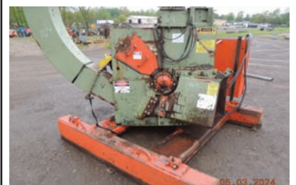
7148 $32,500.00 CHIPPER 48" 6 knife chip-pac, includes 5' x5' shaker screen, electric drive, includes soft start, numerous spare knives and parts, good working condition 260-633-4047
