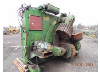
6045 RING DEBARKER $57,500.00 30" dia Cambio ring debarker, 6 arms, steel infeed press wheels, all electric, all electrical and controls included, recently in production and in good working condition, infeed/ outfeed also available, call for price 260-633-4047
