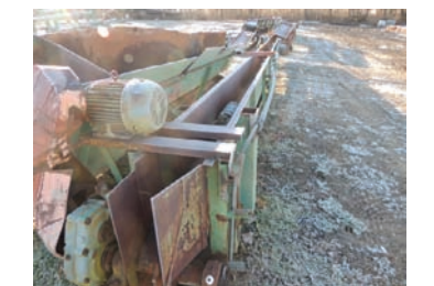
9142 $8,500.00 WASTE CONVEYOR 10"x60' waste conveyor H78 chain with paddles, electric drive ,includes new chain 260-633-4047
