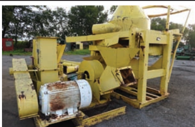
7154 $22,500.00 CHIP-PAC Fulghum 48" dia chipper, 3 knives, 150 hp electric drive, 5' x5' shaker screen-electric drive, chip blower-electric drive, complete unit that is in good condition and ready to work 260-633-4047
