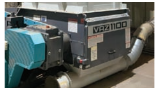
2023 Vecoplan VAC 1100 Grinder Shredder — Specifications & Features — Make: Vecoplan. Model: VAC 1100 XLXR. Serial #: 18876-010. Drive Type: Electric. Includes Blower: no. Teeth Type: Removable 4-sided teeth. Capacity: 42" x 50" top opening. Feed: Top. — Seller Statement — One owner machine, new in 2023, 60 hp electric motor, hyd push cylinder feed, including plastic surround above hopper. Includes Support tools. In great condition, a must have machine! Rigging or Loading fee wil apply
