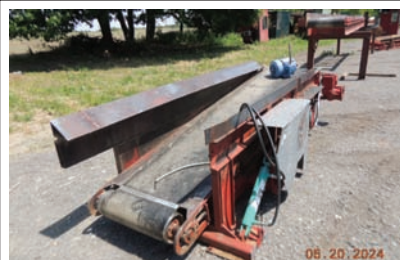
9180 $6,500.00 SLAB DROP BELT 24" wide x 12' long, electric drive, hyd cylinder for drop belt, includes hyd unit for cylinder, very good condition 260-633-4047
