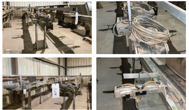
Optimizing Saw Outfeed — Description — 8" x 30' belt, air cylinder, kickers, for parts. Eligible for free loadout
