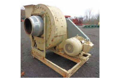
10384 $3,500.00 AMW DUST BLOWER 60" dia housing, 24" inlet/ 18" x 21" outlet, 100 hp electric motor power, good condition, 2 units available 260-633-4047 Wolcottville, IN
