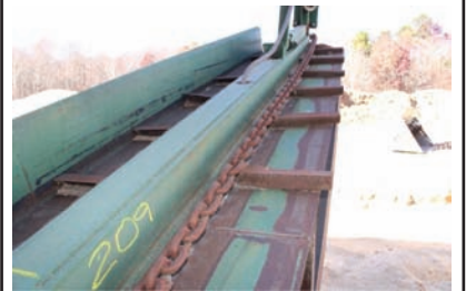
10395 $6,500.00 WASTE CONVEYOR Cornell style chain waste conveyor, 10" wide paddles, 10' flat section and 30' long incline section, electric drive, good working condition 260-633-4047 Wolcottville, IN
