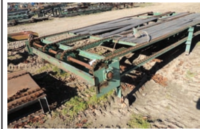
9249 $5,000.00 TRANSFER DECK 4 strand, 10' wide x 22' long, H-78 chain, good condition 260-633-4047
