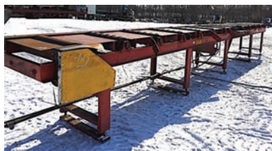
9362 $4,500.00 MELLOTT ROLL CASE 24" wide x 26' long, 6 1/2" dia rollers, has air powered stop & spiral rolls, electric drive, good working condition 260-633-4047 Wolcottville, IN
