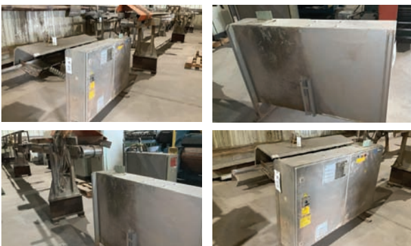
Optimizing Saw Outfeed — Description — 9" x 36', air cylinder board kickers, no belt, includes electrical control box. For parts. Eligible for free loadout
