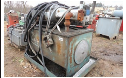
18224 $2,000.00 HYD POWER UNIT 15 hp electric power, vane type pump, includes 4 electric valves, approx 60 gal capacity, very good condition 260-633-4047
