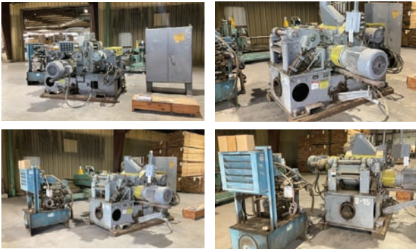
Yates-American Planer — Specifications & Features — Make: Yates American. Model: B-15. Serial #: B-29588. — Seller Statement — Double Head planer, 4" x 16" capacity, spiral indexing bit heads, hyd feed, includes hyd Pak with no motor. Electrical box. Extra parts. Eligible for free loadout
