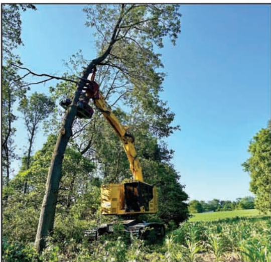
Topping the tree can help minimize damage to the residual stand—in this case it saved the stand of corn.
