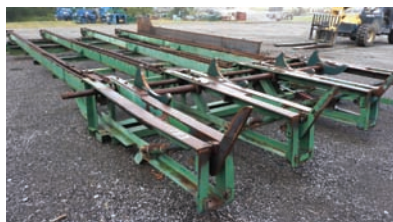
9321 $10,500.00 LOG DECK Edmiston log deck, 4 strands 12" wide x 34' long H-78 chain, stop-load, good working condition 260-633-4047
