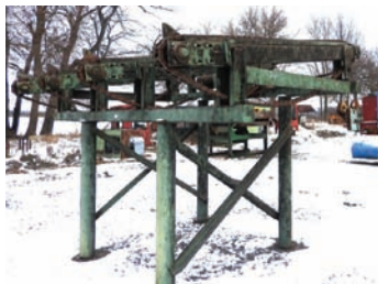
9358 $3,250.00 TRANSFER DECK 4 strand transfer deck, 10' wide x 10' long, H-78 chain, electric gearbox drive, good condition 260-633-4047
