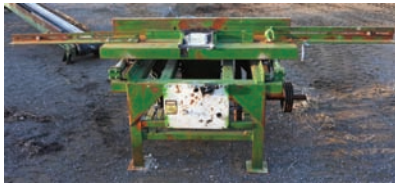
14093 $6,000.00 SINGLE HEAD NOTCHER air powered, line shaft ready, indexable head, working condition 260-633-4047
