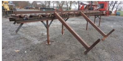
9349 $2,500.00 ROLL CASE 16" wide x 19' long, 4 1/2" dia rollers, dead rolls, roll spacing 11", good working condition 260-633-4047
