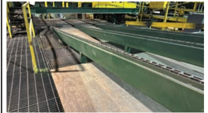
9350 $10,500.00 TRANSFER DECK 3 strand transfer deck, 8' wide x 62' long, 81X chain, electric drive, heavy duty and in good condition 260-633-4047
