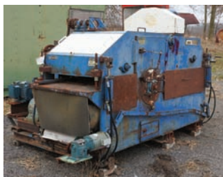
4042 $30,000.00 GANG SAW Quality Machine single arbor gang saw, 6" thick x 24" wide capacity, has indexable sized head, waste belt, all electric drive, 100hp, 25hp, and 10hp motors, 10 blades and lots of various spacers, has 6' in feed, good working condition 260-633-4047
