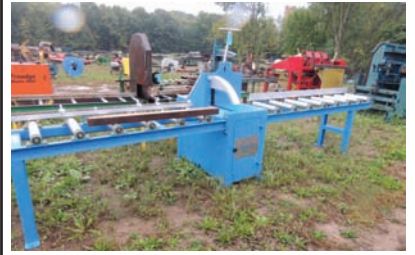
17094 $10,781.00 PROCUT CHOP SAW up-cut style, 7" x9" cutting capacity, 22" dia blade, includes 8' infeed/outfeed, 4 flip stops, BRAND NEW, buy this one or order one to your specs 260-633-4047
