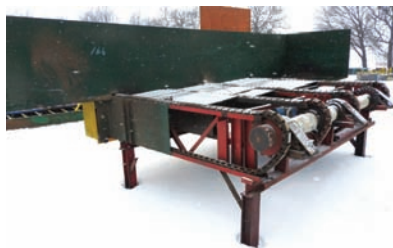
9355 $4,500.00 TRANSFER DECK 4 strand transfer deck, 8' wide x 12'-6" long, H-78 rooftop chain, electric drive, good condition 260-633-4047
