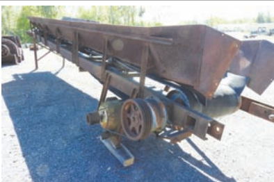
9325 $4,500.00 BELT CONVEYOR concave style belt conveyor, 30" wide x 27' long, electric drive, working condition 260-633-4047
