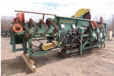
17099 $27,500.00 MERCHANDISING SAW Compact Maxi-Tour merchandising saw system, 72" dia blade, 75 hp electric drive, includes infeed/outfeed conveyors, 260-633-4047
