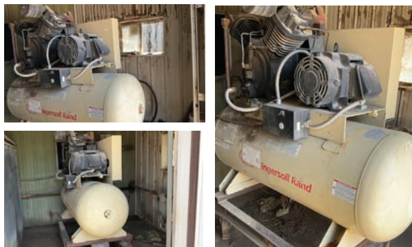
Ingersoll Rand 7100E Air Compressor
