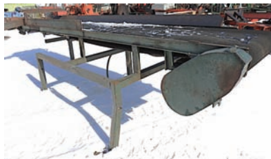
9360 $2,750.00 BELT CONVEYOR 30" wide x 14' long, electric drive, approx 5" tall sides, good working condition 260-633-4047
