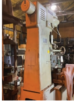
Cleereman Vertical Jig Borer — Description — 16" x 36" table, drilling & milling machine.
