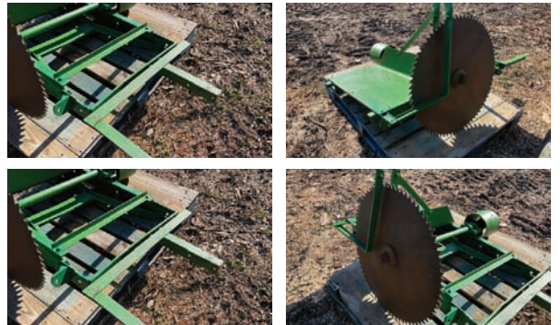
Buss Saw — Description — Tractor front mount cutoff saw. 30" blade. — Contact — Specialist: Dale Nissley, 574-821-6014.
