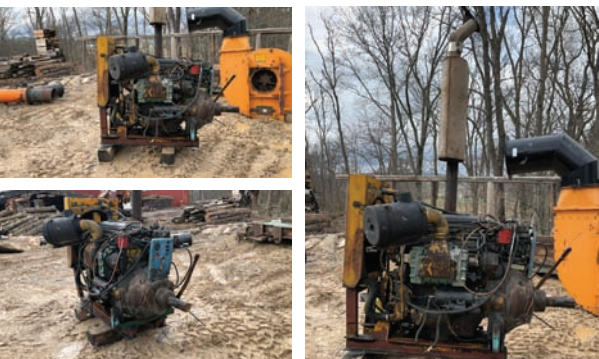
Detroit Diesel Power Unit — Specifications & Features — Year: na. Make: Detroit. Model: 471. Serial #: na. Engine Cylinder: 6.0. Fuel: Diesel. Meter Reads: 3,436. Horsepower: 110. Voltage: 12. Clutch: yes. — Seller Statement — Actual hours unknown, radiator has a small leak, air compressor on the engine need to be rebuilt, engine in itself works good, will use some oil. — Contact — Specialist: Dale Nissley, 574-821-6014.
