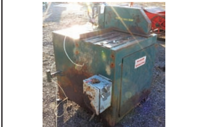
17130 $3,000.00 CHOP SAW up cut chop saw, 10 hp electric motor, air cylinder for blade up-down movement, 20" blade, working condition 260-633-4047
