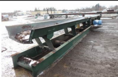
9119 $13,750.00 VIBRATING CONVEYOR Jeffrey vibrating conveyor, 18" wide pan x 36' long, 6" tall sides, electric drive, good working condition 260-633-4047
