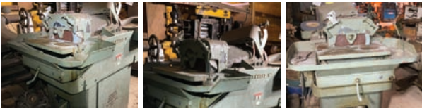
Hammond Dual Wheel Grinder — Specifications & Features — Make: Hammond. Model: 14-W. Serial #: 4362. — Seller Statement — 14" wheels, 3 hp . 3 phase. Tilting tables.
