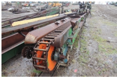
9063 $14,300.00 LOG TROUGH 30' long, 12" wide ladderback chain, electric gear box drive, 1 set of log kickers, good condition 260-633-4047
