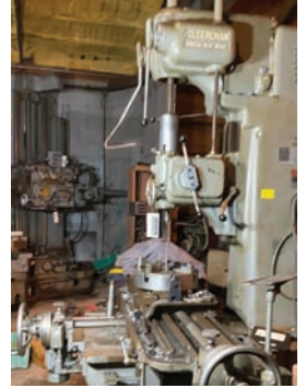
Cleereman Vertical Jig Borer — Description — 16" x 36" table, drilling & milling machine.
