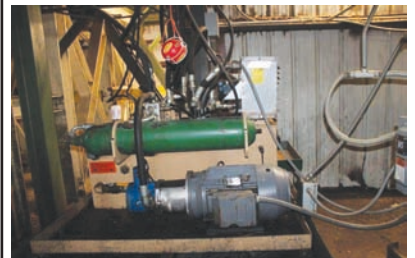
8066 LOG TURNER $7,500.00 Sering bar type log turner, 48" arm, hyd drive, includes 50 hp electric powered hyd unit, good working condition 260-633-4047
