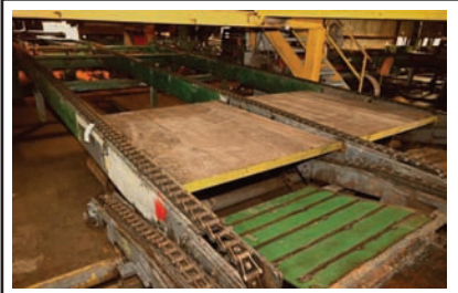
9031 $8,000.00 TRANSFER DECK 3 strand transfer deck, 11'6" wide x 28' long, electric drive, H-78 chain, good condition 260-633-4047
