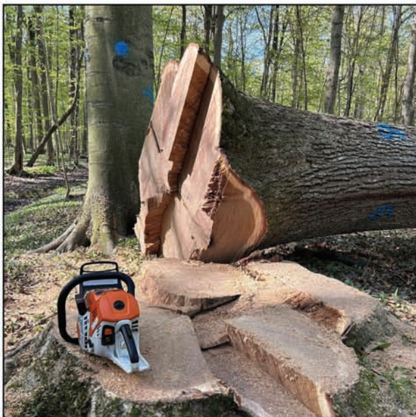
This veneer White Oak was cut with the tongue-and-groove technique.
