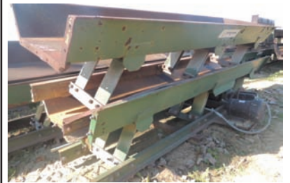
9065 $14,300.00 VIBRATING CONVEYOR Progress 24" wide pan x 35' long, 9" sides, good condition 260-633-4047
