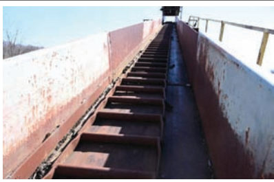
9024 $7,500.00 CHAIN CONVEYOR 15" ladder back chain, 24" pan, 16" sides, 32" x 53' electric drive, good condition 260-633-4047
