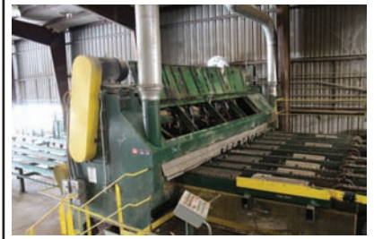
17127 $45,000.00 DROP SAW TRIMMER Newnes drop saw trimmer, 16' long capacity, 9 saws, 75 hp electric motor single drive unit for all saws, easy to set up for line-shaft, air power for heads up/down movement, includes infeed deck/ even-end rollers, includes control station, good working condition 260-633-4047
