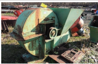
10351 CHIP BLOWER $4,250.00 36" dia chip blower, single chip loading chute, outlet 12" x 14", 25hp electric drive, good working condition 260-633-4047
