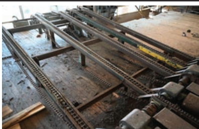
9018 TRANSFER DECK $4,600.00 5 strand, 13' wide x 18' 6" long, H78 chain, electric drive, air cylinders on pop up board stop, good condition 260-633-4047
