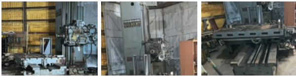
Cincinnati Gilbert Mill — Description — Horizontal mill, 78" x 53" moving table, 6' vertical movement, digital controls
