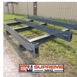
9085 $24,500.00 SUPREME MFG LOG DECK 3 strand 10' wide X 20' long log deck, Tulsa Winch electric drive, H-78 chain, heavy duty built. BRAND NEW! 260-633-4047
