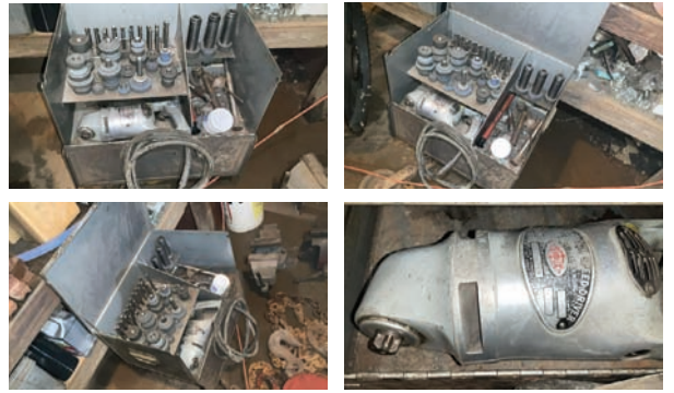
Portable Valve Grinder Kit — Description — Large assortment of bits, in metal storage case . handheld high-speed grinder.
