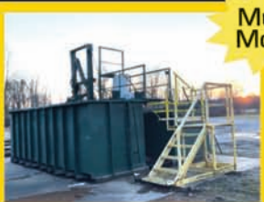
Lumber Dip Tank
