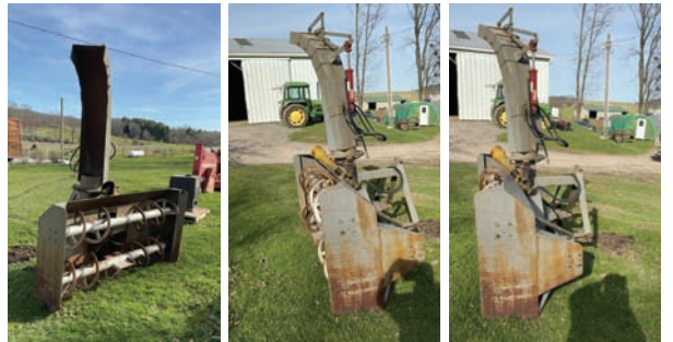
Tractor Mounted Snow Blower — Description — 86" wide, 3 point hitch and pto attachment
