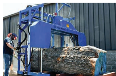
1636 $45,000.00 TRU CUT EHS 70 BAND MILL 2022 model. Equipped with 2" band, 28" band wheels, and hydraulic band tensioning, 70" diameter cutting capacity with 55" total blade height movement. Includes electric motor, sawdust chute, and exhaust port. Call for details. Make your offer today! 281-541-3980
