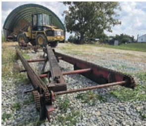
9632 3-STRAND LOG DECK $4,500.00 3-Strand Log Deck - 25' long, equipped with a Tulsa gearbox powered by a hydraulic motor. In good working condition and ready to be put back into service. A solid log-handling addition for your mill operation. Call for details and make your offer today! 502-905-1940
