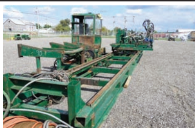
2087 $20,000.00 HMC 4 HEAD BLOCK CARRIAGE HMC HC-40, serial #330-1982, 4 head-block carriage, 110 volt electric over air set-works, 50 hp carriage drive, air powered dogs, 40' long track, was used with band head, includes cab, controls and log turner, complete unit ready to operate and in good condition 260-633-4047
