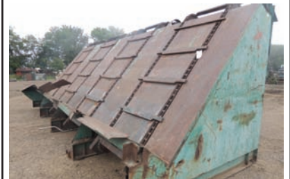
9020 $9,750.00 UNSCRAMBLER 4 strand, 33" slats on each strand, electric drive, unit is 80" tall, good condition 260-633-4047
