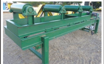
9217 $4,500.00 ROLL CASE pop-up rollers, perfect for putting in a transfer deck, 16" wide x 7' long, foot pedal control, hyd drive, BRAND NEW! 260-633-4047
