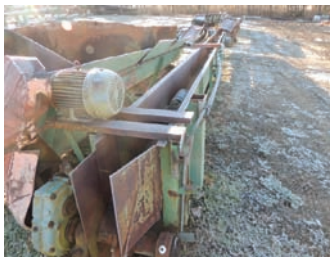
9142 $8,500.00 WASTE CONVEYOR 10"x60' waste conveyor H78 chain with paddles, electric drive ,includes new chain 260-633-4047
