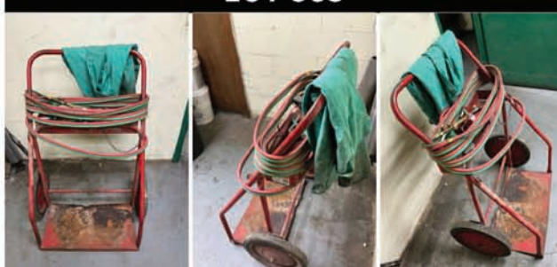
Continental & Radnor Oxy-Acetylene Welding Cart Setup with Torch and Hoses
