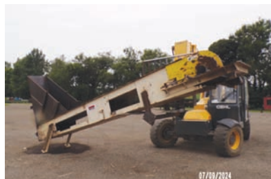
9206 $3,500.00 CLEATED BELT CONVEYOR 24" wide x 18' long, set up for incline, electric drive, excellent condition 260-633-4047
