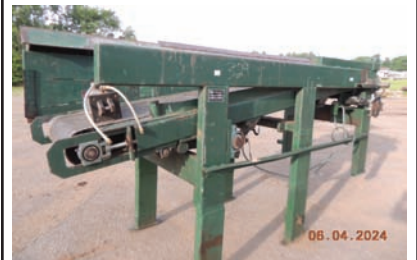
9191 $9,500.00 PENDU SLAB DROP BELT 24" wide x 10' 6" long, hyd drive, twin air cylinders for up-down on belt, heavy duty and in excellent condition 260-633-4047
