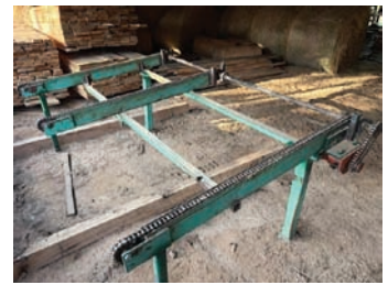
9304 $2,500.00 TRANSFER DECK 3 strand transfer deck, 8' wide x 7' long , hyd drive, good working condition 260-633-4047
