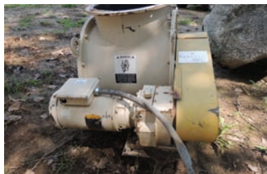
10275 $4,000.00 AIR LOCK Koger-Air, 14" dia inlet/outlet, electric drive, very good condition 260-633-4047
