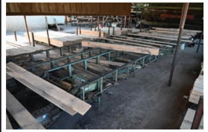
9380 GREEN CHAIN $11,500.00 4 strands 10' 6" wide x 53' long, electric drive, C-55 rooftop chain, good working condition 260-633-4047
