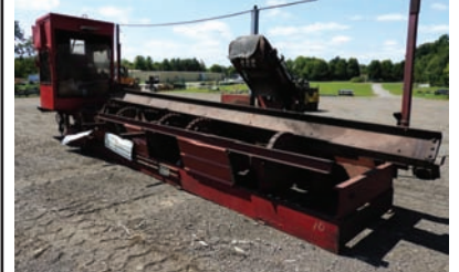
6046 DEBARKER Mellott rosser-head debarker, your choice of power (electric or hyd), new babbit in bearings, new cleats on bull wheels, good condition and ready for production 260-633-4047
