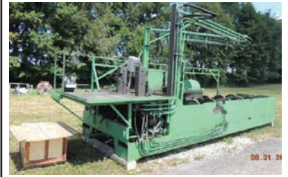
6031 HMC DEBARKER rosser head style, all hyd. drive, 36" dia. log capacity x 12' long, very good condition 260-633-4047
