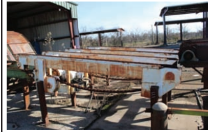
9267 $3,750.00 TRANSFER DECK 4 strand transfer deck, 10' wide x 11' long, 5 hp electric gear-box S style drive, 81X chain, heavy duty and in good working condition 260-633-4047
