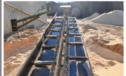
10394 $8,500.00 WASTE CONVEYOR Cornell style chain bran sweep, 14" wide paddles, 27' flat section, 30' long incline section, electric drive, good working condition 260-633-4047
