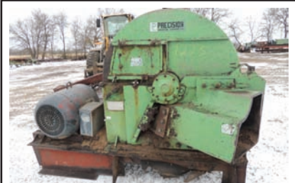
7109 PRECISION CHIPPER 48" dia. 6 knife wheel with 3 blocked, bottom discharge, good condition 260-633-4047
