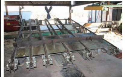
9383 TRANSFER DECK $5,500.00 6 strand transfer deck, 10' 6" wide x 16' long, C-55 rooftop chain, electric drive, good working condition 260-633-4047
