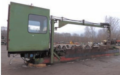
6044 DEBARKER Mellott rosser-head debarker, electric drive, hyd cylinder for head up-down, recently in production and in good operating condition 260-633-4047
