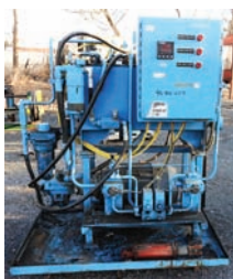
18250 HYD UNIT $4,500.00 30 HP electric, approx 60 gal tank, pressure comp pump system, includes electrical panel and several valves, excellent condition 260-633-4047
