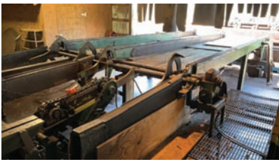
9387 $8,750.00 LOG DECK 3 strand log deck, 10' wide x 24' long, hyd Tulsa winch drive, stop-load arms, H-78 chains, good working condition 260-633-4047
