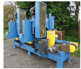
3098 $25,000.00 RESAW West Plains 2 head resaw, 6" wide capacity, electric drive, block guides, recently in production and ready to work 260-633-4047
