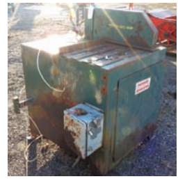
17130 $3,000.00 UP CUT CHOP SAW 10 hp electric motor, air cylinder for blade up-down movement, 20" blade, working condition 260-633-4047 Wolcottville, IN
