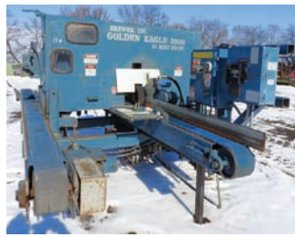
3093 $15,000.00 RESAW Brewer Golden Eagle single head resaw, electric drive, 36" dia wheels, return belt, includes numerous extra blades, this machine is in excellent condition and ready for production 260-633-4047
