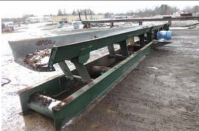
9119 $13,750.00 JEFFREY VIBRATING CONVEYOR 18" wide pan x 36' long, 6" tall sides, electric drive, good working condition 260-633-4047
