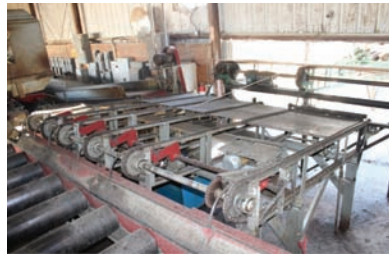
9382 TRANSFER DECK $3,750.00 6 strand transfer deck, 10' 6" wide x 11' long, C-55 rooftop chain, electric drive, air stops on one end, good working condition 260-633-4047
