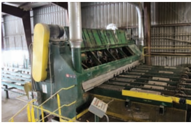
17127 $45,000.00 DROP SAW TRIMMER Newnes drop saw trimmer, 16' long capacity, 9 saws, 75 hp electric motor single drive unit for all saws, easy to set up for line-shaft, air power for heads up/down movement, includes infed deck/ even-end rollers, includes control station, good working condition 260-633-4047 Wolcottville, IN
