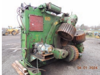
6045 RING DEBARKER 30" dia Cambio ring debarker, 6 arms, steel infeed press wheels, all electric, all electrical and controls included, recently in production and in good working condition, infeed/ outfeed also available, call for price 260-633-4047
