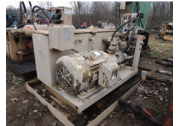
18153 $4,000.00 GS HYD. UNIT 25 HP. electric drive, 2 pump sections, one is a pressure compensated, very good condition 260-633-4047 Wolcottville, IN
