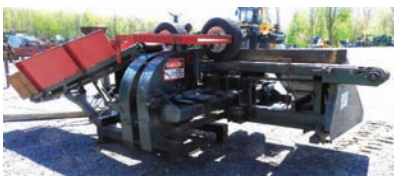
3105 $32,500.00 RESAW Baker 3- head band resaw, set up for line-shaft operation, upgraded to guide rollers, includes "built-in" cant sizer, good working condition 260-633-4047
