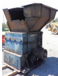
7174 $9,500.00 JEFFERY WASTE GRINDER top feed opening is 27" x 33", swinging hammer style, bottom discharge, working condition 260-633-4047 Wolcottville, IN
