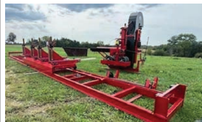
1664 $75,000.00 2026 PERFORMAX BAND MILL Brand new, right-hand mill with 2" bands and 42" wheels, 42" handset, and a 16' 4-headblock all-manual carriage with Timber Buddy heavy-duty wheels. Includes 45' track, 39" throat, and weight strain. Write to: Chris Mast, 19655 State Hwy DD, Newtown, MO, 64667. Make an offer today! 574-536-1646
