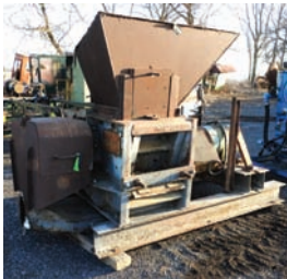
7173 $7,500.00 WASTE GRINDER Williams crusher/ pulverizer, swinging hammer style, 25 hp electric drive, top feed 15" x 18", bottom discharge, working condition 260-633-4047 Wolcottville, IN
