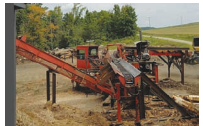
6610 $45,000.00 MORBARK 636 DEBARKER PACKAGE Complete hydraulic debarker setup with a 14' infeed log deck, 18' ladder-chain log trough, and mulch chain conveyor underneath with incline discharge. All hydraulics are in good working condition. Power unit is not included but is available as an option to purchase. Ready for production. Call for details and make your offer today!
