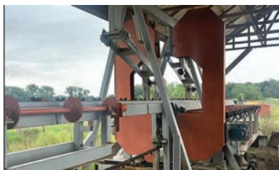
1663 NEW TWIN BAND SCRAGG MILL Equipped with 26" Cook's band wheels, sharp-chain feed, and Echo networks, adjustable for logs approximately 5"-12". Excellent for producing pallet cants and cut stock. Includes a log roller/turner. Simply connect your hydraulics and it's ready to cut! Call or check the full-page ad in the magazine. 240-925-4232
