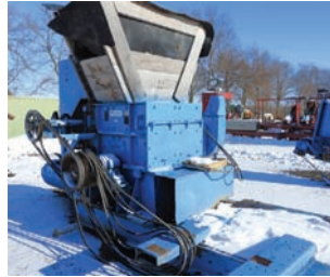
7171 $12,500.00 JEFFREY 44 WB-HOG Jeffery waste grinder, top feed opening is 44" wide x , swinging hammer style, includes blower and infeed belt conveyor, blower and belt are hyd powered, good working condition 260-633-4047 Wolcottville, IN
