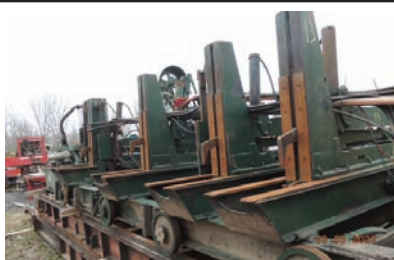
2078 $47,500.00 CLEEREMAN 4 HB MILL Cleereman 4 head block, Model 40, air over air setworks, includes cab/track-frame/ carriage drive and all controls, in good working condition. 64' track length, 16' carriage 260-633-4047
