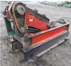
8059 $4,200.00 LOG TURNER chain type log turner, 36" chain, hyd drive, good working condition 260-633-4047
