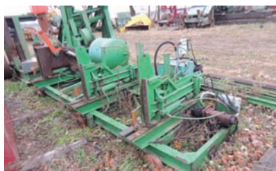
2063 $35,000.00 CIRCLE MILL Cleereman 3 head-block, 36" carriage, Timber Tiger electric set-works, includes track/ drive/ 60" husk/ cab and all controls, in good working condition 260-633-4047
