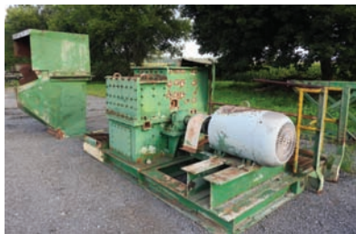
7155 $8,500.00 PROGRESS WASTE GRINDER swinging hammer style, 125 hp electric drive, 1185 rpm's, unit needs to have hammers installed, good overall condition 260-633-4047
