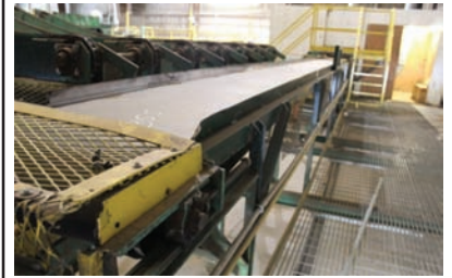
9343 BELT CONVEYOR $4,500.00 24" wide x 30' long, hyd drive, approx 4" tall sides, good condition 260-633-4047
