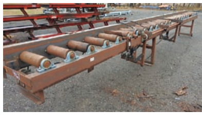
9348 ROLL CASE $2,500.00 14" wide x 25' long, 4" dia rollers, rolls spaced every 8", hyd drive, good working condition 260-633-4047
