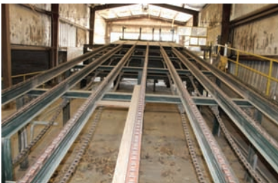
9344 TRANSFER DECK $7,500.00 7 strand transfer deck, 12' wide x 45' long, 81X chain, electric drive, good working condition 260-633-4047
