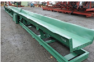
9347 VIBRATING CONVEYOR $15,500.00 24" wide pan x 46' long, approx 9" tall sides, hyd drive, good working condition 260-633-4047
