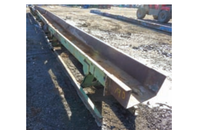
9226 VIBRATING CONVEYOR $15,000.00 Precision vibrating conveyor, 18" wide pan x 55' long, 8" sides, electric drive, good working condition 260-633-4047
