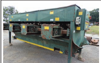
17114 $27,500.00 TRIM SAW 4 head trim saw with electric powered head adjustment, 6" x 12' long capacity, includes material and waste belts, 9'6" x 16' foot print, price includes going through shop, ready for production 260-633-4047
