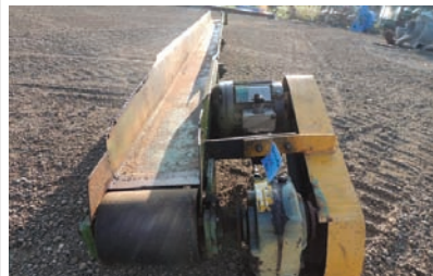
9012 $2,000.00 BELT CONVEYOR 20" wide x 20' long, 7" sides, electric drive, working condition 260-633-4047
