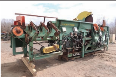
17099 $27,500.00 MERCHANDISING SAW Comact Maxi-Tour merchandising saw system, 72" dia blade, 75 hp electric drive, includes infeed/outfeed conveyors, 260-633-4047
