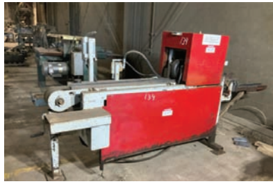
14091 $5,500.00 BOARD DEDUSTER Go-Fast pallet board deduster, hyd drive, 6" wide capacity, good working condition 260-633-4047
