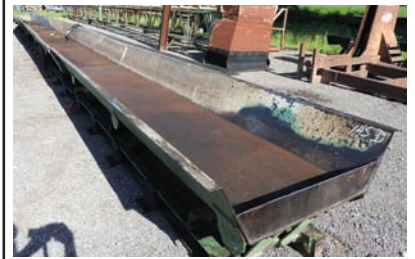
9296 $22,500.00 VIBRATING CONVEYOR Precision vibrating conveyer, 30" wide pan x 58' long, 12" tall sides, hyd drive, excellent condition 260-633-4047
