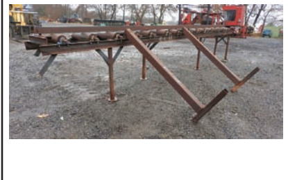
9349 ROLL CASE $2,500.00 16" wide x 19' long, 4 1/2" dia rollers, dead rolls, roll spacing 11", good working condition 260-633-4047
