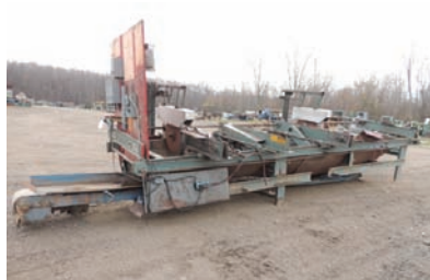
17079 $5,750.00 TRIM SAW Newman K-20 double end trim, 22" blades, electric drive, 16' long capacity, good condition 260-633-4047
