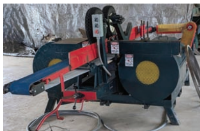
3631 $8,000.00 MORGAN RESAW W/RETURN BELT 15 HP, 480V, 3-phase electric motor. Uses 1" band with cutting capacity up to 8". Equipped with 6" non-slip vari-drive feed belt and spring-loaded hold-down wheels. Overall dimensions: 11' long, 68" wide, 52" high. Total weight approx. 1,650 lb. In excellent condition. Make your offer today! 607-642-8355
