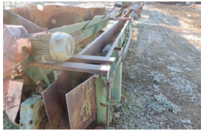
9142 $8,500.00 WASTE CONVEYOR 10"x60' waste conveyor H78 chain with paddles, electric drive .includes new chain 260-633-4047
