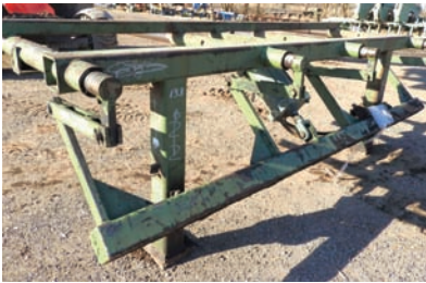
9244 CANT CATCHER $8,000.00 Reckart cant catcher for drop use with a drop belt, air powered, 4 arms, travel is 30", good working condition 260-633-4047
