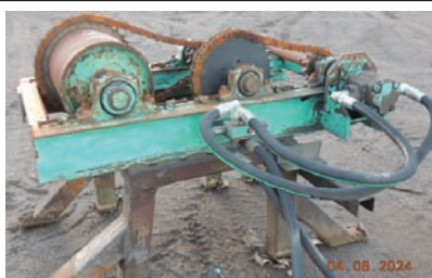
20308 $2,800.00 CARRIAGE DRIVE Helle drum unit for carriage drive, drum is 13 1/2" dia x 16" wide, hyd drive, good working condition 260-633-4047
