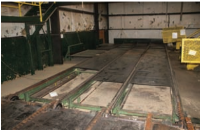
9335 $7,500.00 TRANSFER DECK 10' wide x 40' long, H-78 chain, electric gear-box drive, includes panning in between strands, very good condition 260-633-4047
