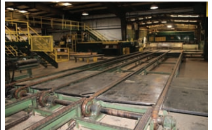
9336 $8,500.00 TRANSFER DECK 5 strand transfer deck, 10' wide x 55' long, H-78 chain, electric drive, good working condition 260-633-4047
