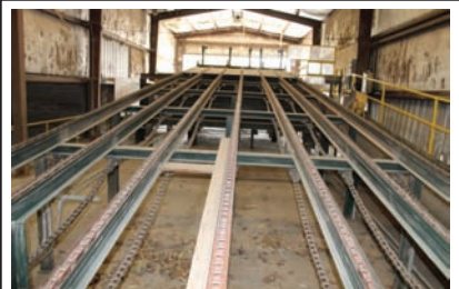
9344 $7,500.00 TRANSFER DECK 7 strand transfer deck, 12' wide x 45' long, 81X chain, electric drive, good working condition 260-633-4047
