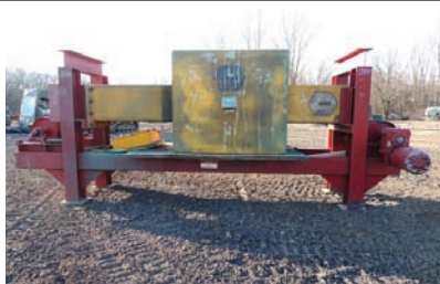
20274 $11,500.00 METAL DETECTOR 18"W belt 22" opening 15' long 74" high, excellent condition 260-633-4047
