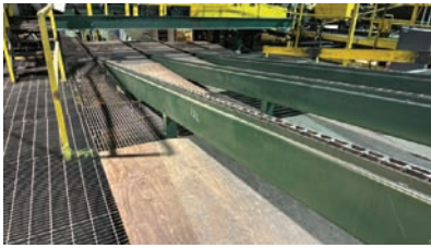
9350 TRANSFER DECK $10,500.00 3 strand transfer deck, 8' wide x 62' long, 81X chain, electric drive, heavy duty and in very good condition 260-633-4047
