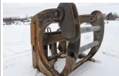
20306 $4,500.00 GRAPPLE FORKS 73" wide overall, pin-on style, 40" center to center on bottom pins, 2-1/4" pins, good working condition 260-633-4047
