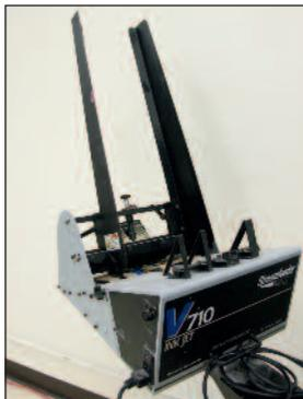
Streamfeeder V710 Ink Jet Friction Feeder
