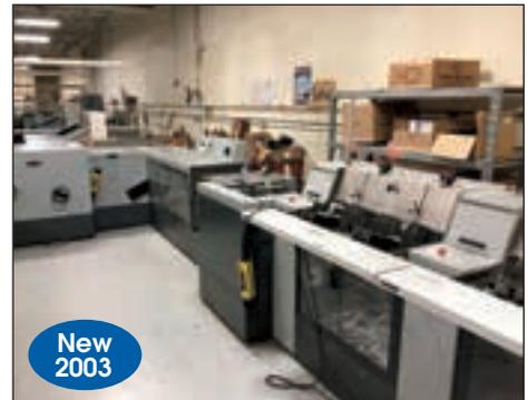
HEIDELBERG SADDLE STITCHER # ST100, 6-PKT COVER FEEDER, SCORING 3-KNIFE TRIMMER, STITCHING HEADS, DELIVERY CONVEYOR
