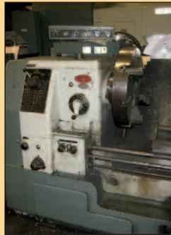
OKUMA # LT ENGINE LATHE (27.5"/35" x 123" Cap.)
