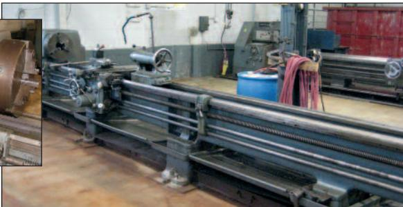
VDF 21" x 240" ENGINE LATHE
