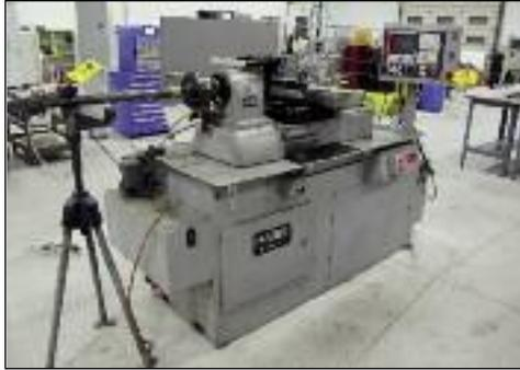
Hardinge #DSM CNC Lathe w/ Fagor CNC Control
