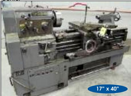
Webb #WL-435 "Gap Type" Engine Lathe
