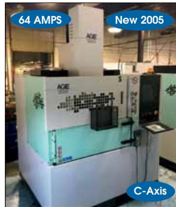
AGIE CNC "Sinker Type" EDM # Agietron-Advance - 3 w/ C Axis
