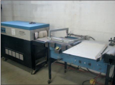
Weldotron Auto Shrinkwrap Machine Model 1602
