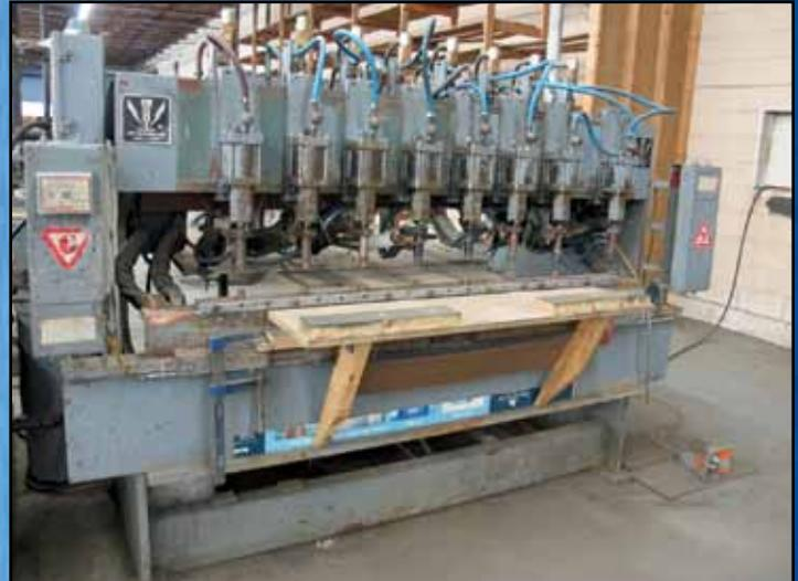
Lors 8-Station Welder Machine MW1 w/ Entron Controls
