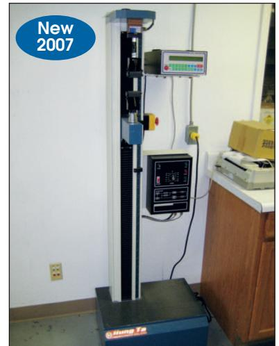
Hung TA Instruments Tensile Tester Model HT8336-S
