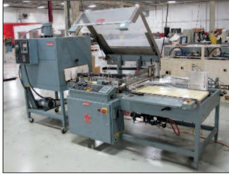
Shanklin #27A L-Seal Packaging Machine w/Heat Tunnel
