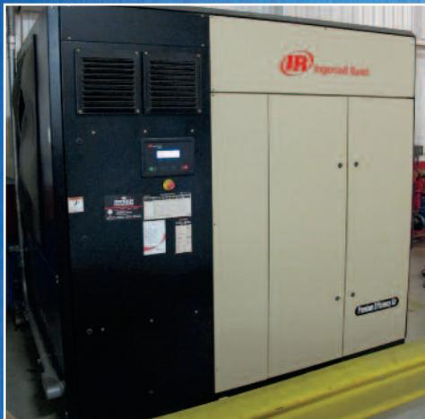
Ingersoll Rand 125 HP Rotary Screw Air Compressor #IRN125H
