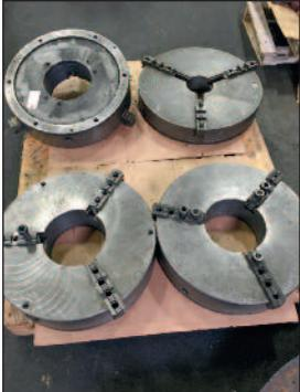
VIEW of "LARGE BORE" 3-Jaw Chucks
