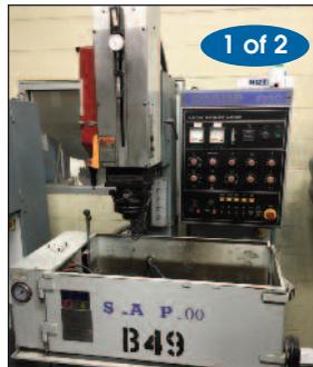
SHARP # F-25C EDM HOLE "Popper-Sinker Type"
