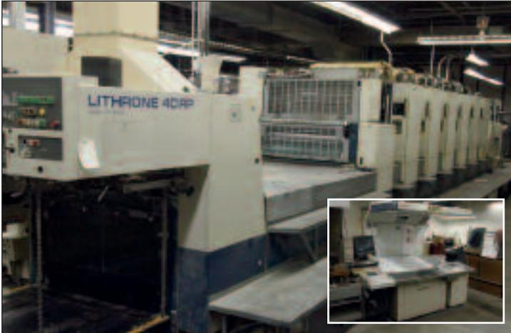
Komori L640RP-III Sheet Fed Printing Press / Komori L640RP-III Console
