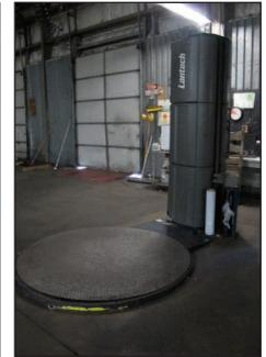
LANE TECH Q SERIES ROTARY STRETCH PALLET WRAPPER
