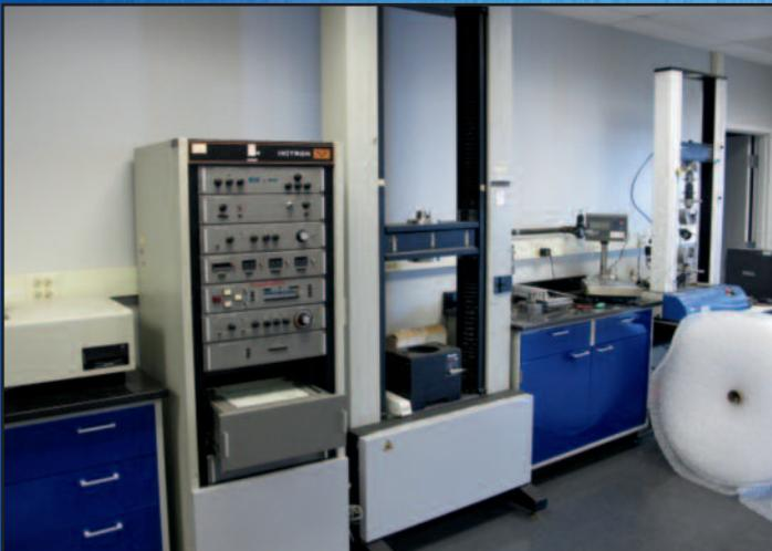
Instron Load Cell Tensile Tester Model 1125
