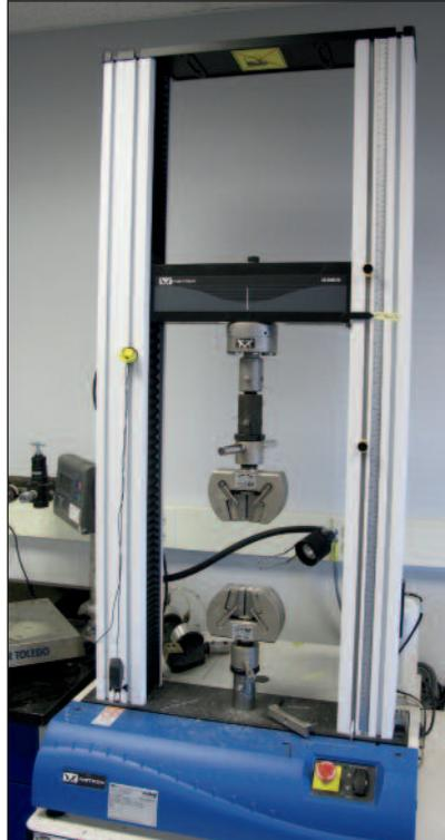
INSTRON LOAD CELL TENSILE TESTER MODEL 3369
