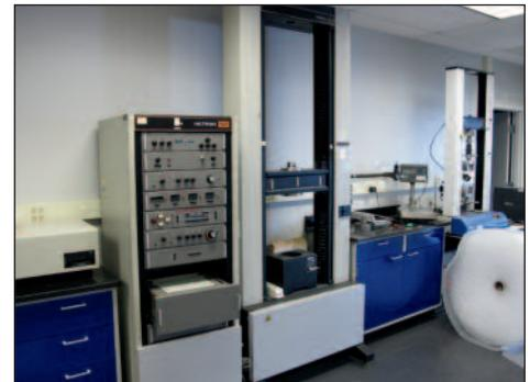
INSTRON LOAD CELL TENSILE TESTER MODEL 1125
