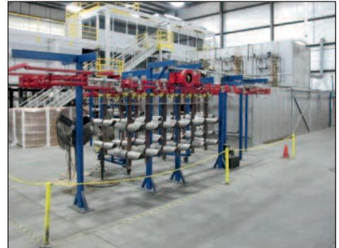
OVEN/DRYING CONVEYOR SYSTEM, 3-LANE OVEN, 230-280 DEG F TEMP
