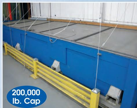
Navtec Hydraulic Pull Tester 200,000 lb. Cap.
