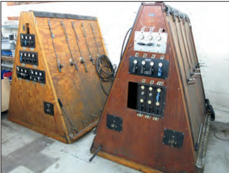
(2) NAVTEC A-FRAME HYDRAULIC PRESSURE TESTERS
