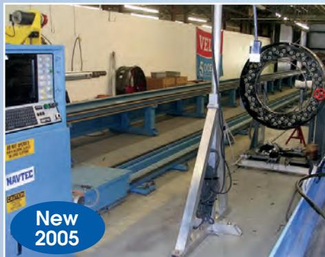
Navtec Fiber Winding Machine
