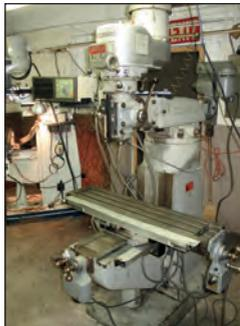
Bridgeport "Series II", 2 HP Vertical Milling Machine
