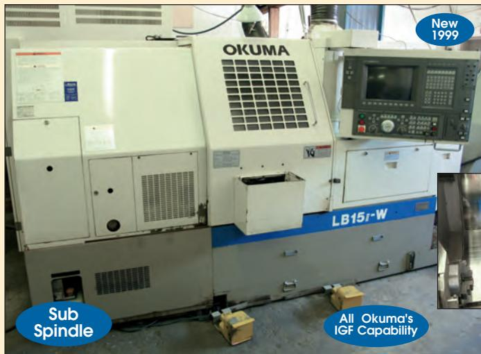
Okuma # LB-15-II-W CNC Turning Center W/ Sub-Spindle
