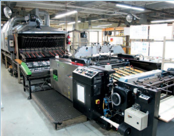
SPS SHEET FED SCREEN PRINTING LINE, VITESSA-FLEX S1-PE
