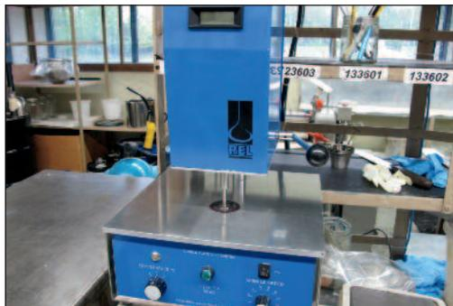
RESEARCH EQUIPMENT CONE & PLATE VISCOMETER
