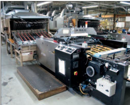
SPS SHEET FED SCREEN PRINTING LINE, VITESSA-FLEX S1-PE W/DRYING SYSTEM
