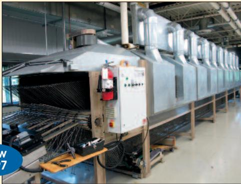
SPS SHEET FED SCREEN PRINTING LINE, VITESSA-FLEX S1-PE W/DRYING SYSTEM
