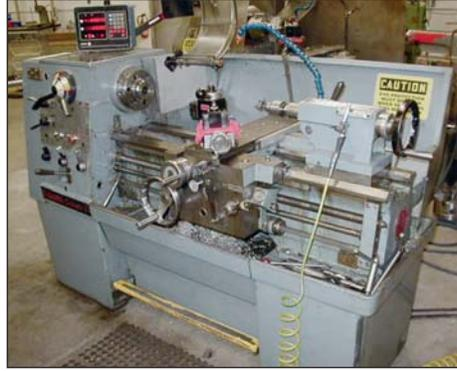
CLAUSING COLCHESTER 15" X 36" ENGINE LATHE
