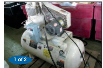
5 HP Horizontal Tank Air Compressor
