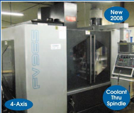
Toyoda FV-965 CNC Vertical Machining Center
