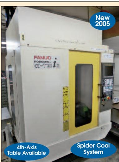
Fanuc Alpha-T211E CNC RoboDrill
