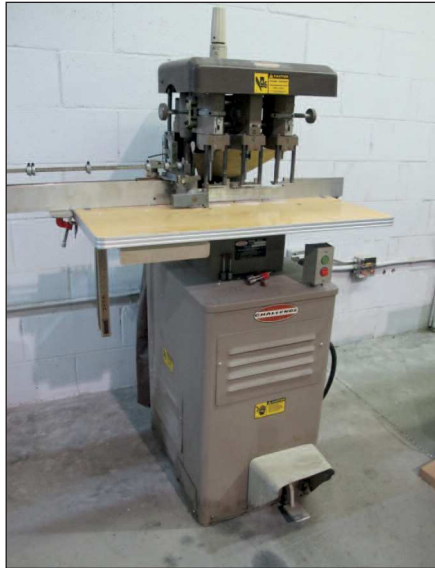
CHALLENGE 3-SPINDLE DRILL MODEL EH3
