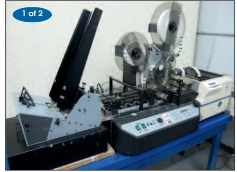
AMERITEK 2000 SERIES TABBING MACHINE W/ SECAP FRICTION FEEDER #FR170
