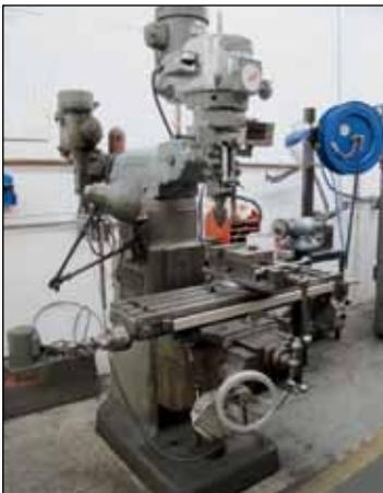
BRIDGEPORT 1.5 HP VERTICAL MILL, POWER FEED
