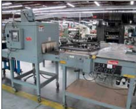
SHANKLIN L-SEAL PACKAGING MACHINE WITH HEAT SHRINK TUNNEL
