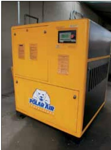
EATON 60 HP ROTARY SCREW AIR COMPRESSOR MODEL EM-RTS3-60
