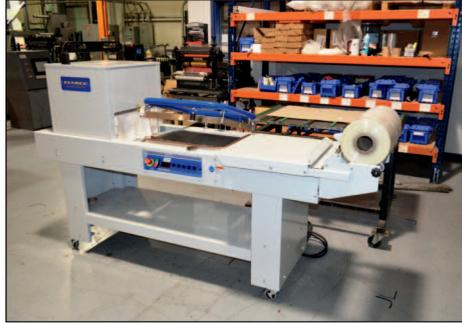
CLAMCO L-SEAL PACKAGING MACHINE MODEL 120-COMBO
