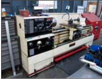
JET LATHE MODEL GH1660ZX, 16" SWING X 60" CC
