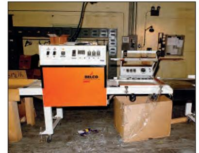
BELCO L-SEAL PACKAGING MACHINE W/HEAT SHRINK TUNNEL
