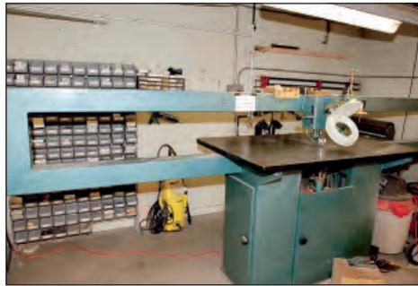
SANDVIK PV185 DIE MAKING JIG SAW MODEL PV1850
