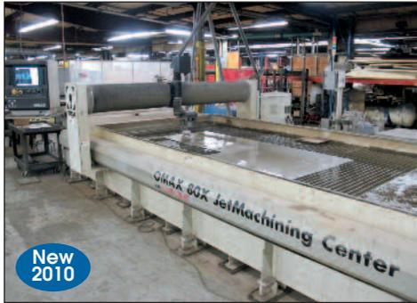
Omax CNC Waterjet System Model 80X
