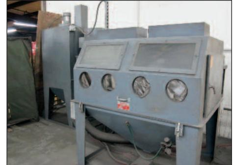
Trinco Mod.# 6044 Dual Station Dry-Blast Cabinet W/Dust Collector
