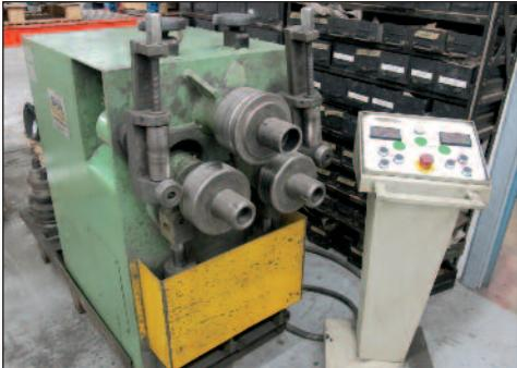
Eagle Tube Bending Machine Model
