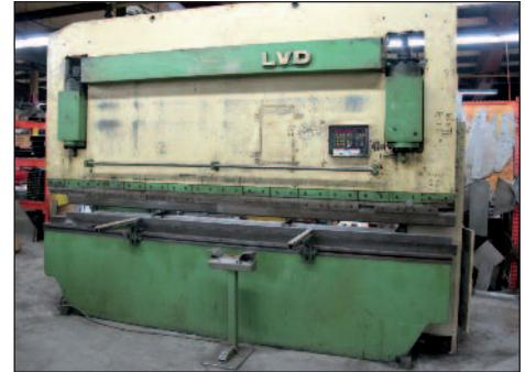
LVD 12' x 200-Ton Hydraulic Power Press Brake Model PPBL200-40
