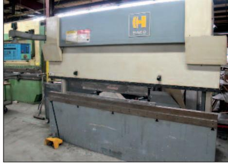
Haco CNC 10' x 120-Ton Euromaster Hydraulic Brake Model SRM-120-10
