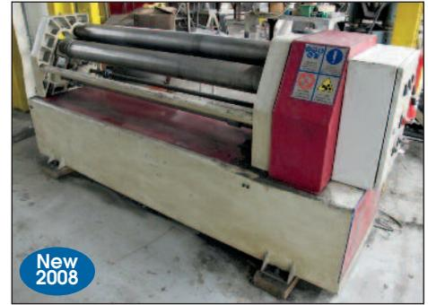
A.K. Bend Bending Rolls Model ASM130-15/4.0mm
