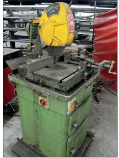
Doringer Model D350 Heavy Duty Cold Saw
