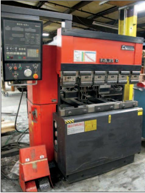
Amada CNC 4' x 35-Ton, Hydraulic Press Brake Model FBD3512E
